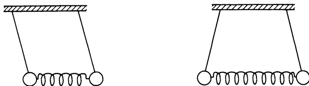
Fig. 10.9. The fundamental oscillations of two coupled pendulums: symmetric and antisymmetric oscillations (normal modes)
