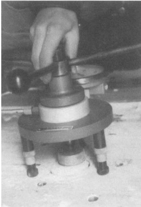
Figure 3-12. Use of the pull-off test; a. , pulling the concrete core; b. , broken core
