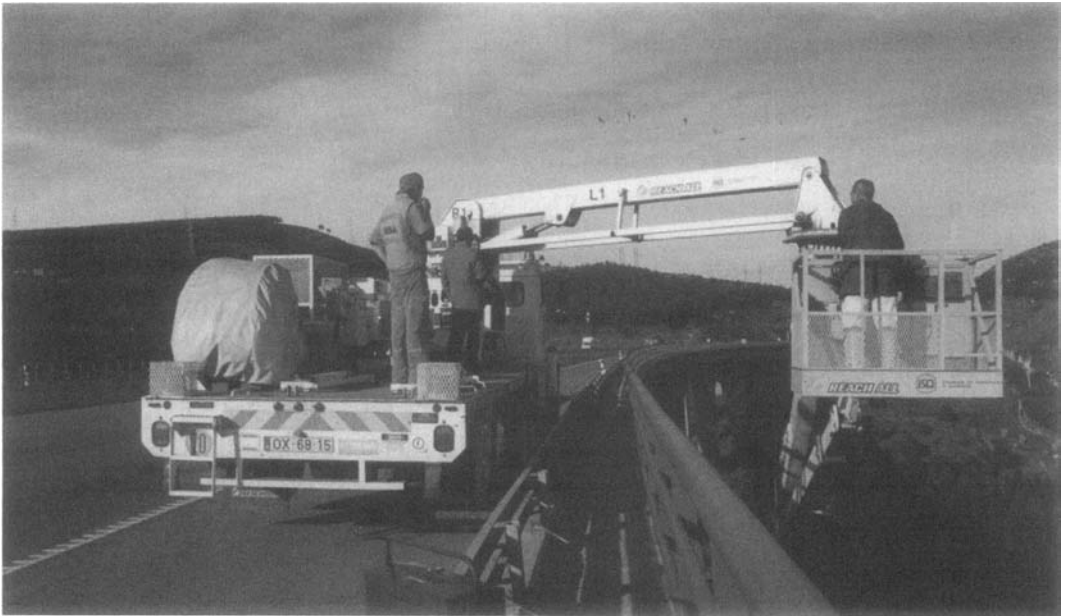
Figure 7-20. Principal inspection vehicle
