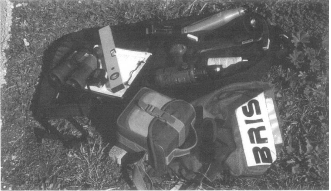
Figure 7-19. Ordinary inspection equipment
