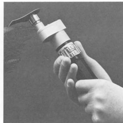
2. Seat attachment over air driver and lock. Run the motor at full speed.
