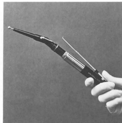
3. Lock bur securely by returning lever flush against attachment.
