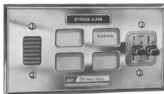
Four-light audio-visual alarm panel combines switch-over Warning Signal (1) and High and Low Main Line Pressure Warning Signals (2a) into a single unit.
