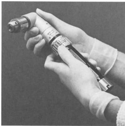
1. Place the attachment over the air driver shoulder. Engage hex drive. Turn ring clockwise to lock.
