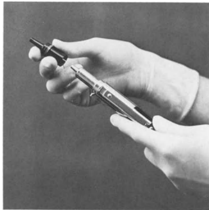
2. Push bur release lever forward 90 degrees to insert the bur. Return lever flush against drill to lock bur.
