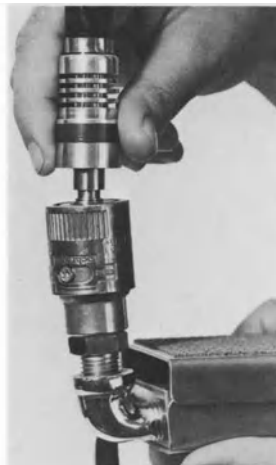
2. Connect the air-drill hose and foot control.
