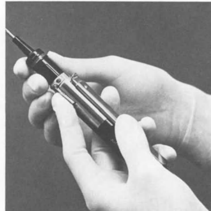
3. Return lever flush against the drill to lock bur.
