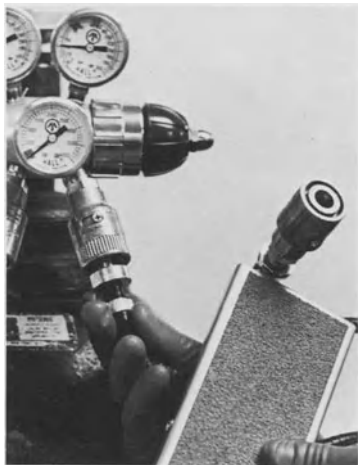
1. Plug the foot-control hose into the regulator.
