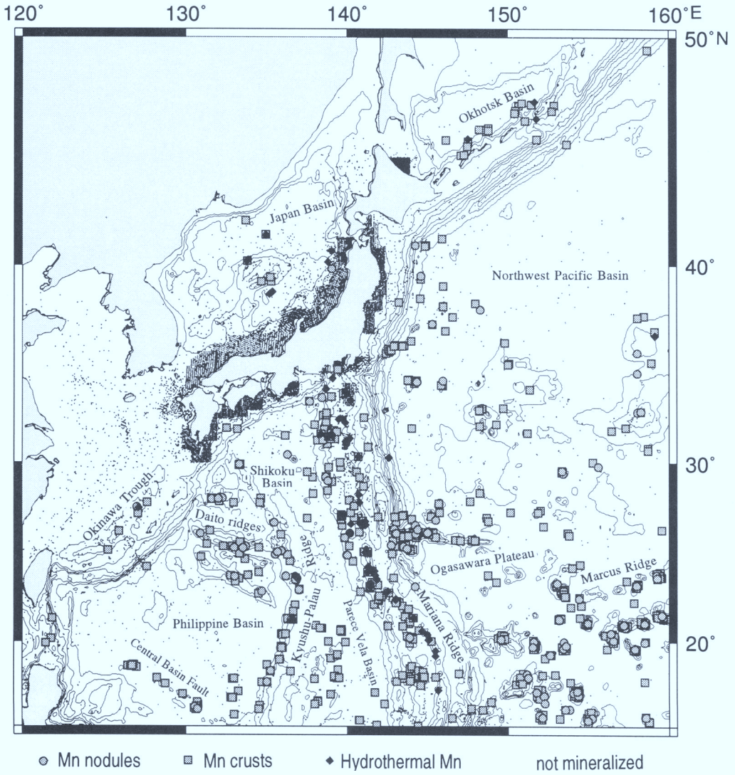
Fig. 4. Occurrence of manganese deposits in relation to topography (contour: 1000 m interval). The plot shows occurrence of manganese deposits whose thickness exceed 1 mm.
