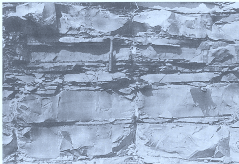
Fig. 5. Thick massive even beds of micritic, siliceous grey limestone (Type a). Note insoluble residue-rich partings or thin beds (Type c) in between thick beds.
