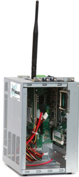
Fig. 8.1: Industrial PC platform and WLAN hardware for the implementation prototype
