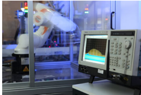
Fig. 3.10: Robot arm (left) with mounted transmitter and the RSA as receiver (right)
