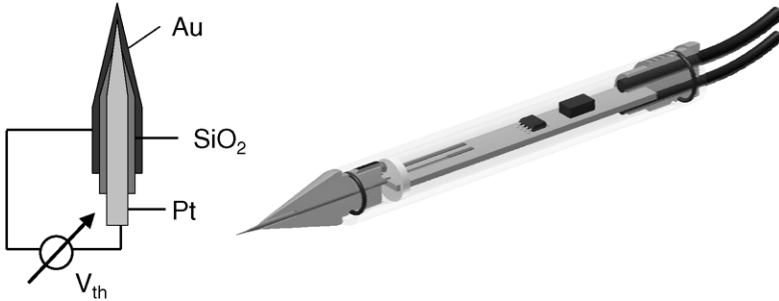
Fig. 2. The basic setup of the thermocouple is shown in the left sketch. The thermocouple is mounted on a tube which serves as a enclosure for the preamplifier as shown on the right.
