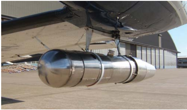
FIGURE 4-6 An airborne ice nucleus generator is shown affixed to an aircraft wing. Such generators consist of three sections: a compressed air tank to provide flow to the liquid seeding solution (front), the solution reservoir (middle), and the combustion chamber (aft). Capacity is typically about 30 L (8 gal.) Source: Courtesy of Jesse Bader.
