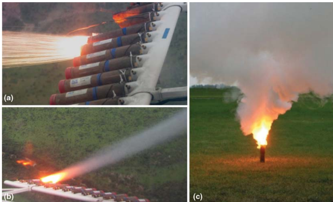
FIGURE 4-5 Hygroscopic calcium chloride pyrotechnics are shown in action. Ignition on an aircraft flare rack is shown in (A), the burn in (B), and for comparison, a ground burn without wind in (C). Each of the flares shown contained 1.00 kg (2.21 lb) of reagent Source: (A) and (B) courtesy of Christopher L. Grilliot; (C) courtesy of James Gunkelman.
