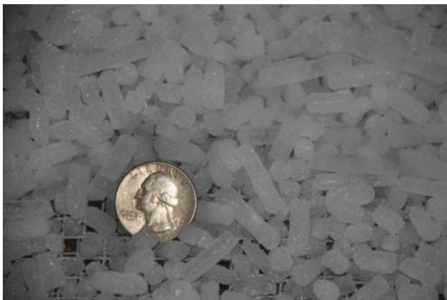
FIGURE 4-4 Dry ice, in extruded pellet form. The pellets shown, of varying lengths, are about 0.6 cm (0.25 in.) in diameter Source: Courtesy of Brook Mueller.
