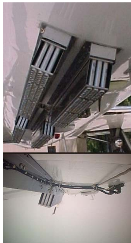
FIGURE 4-3 Racks for ejectable glaciogenic pyrotechnics are commonly mounted on the aircraft belly (top). These flares are 20 mm (0.79 in.) in diameter, and each typically contains 20 g (0.04 lb) of nucleant and binder. When fired, only the flare candle leaves the aircraft (bottom); the aluminum casing remains in the rack
