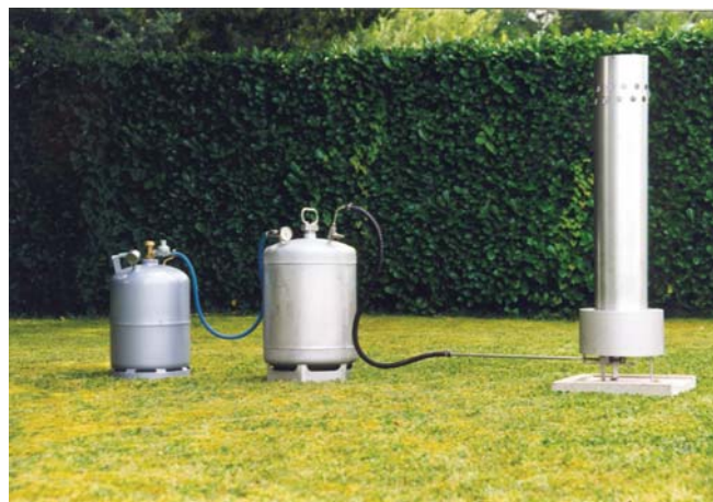
FIGURE 4-7 A ground-based ice nucleus generator used for hail suppression efforts in the French Anelfa program Source: Courtesy of Claude Berthet, Anelfa.
