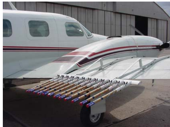
FIGURE 4-2 Glaciogenic cloud seeding pyrotechnics called “burn-in-place” flares are commonly burned in flight, attached to racks affixed to the trailing edges of the aircraft wings
