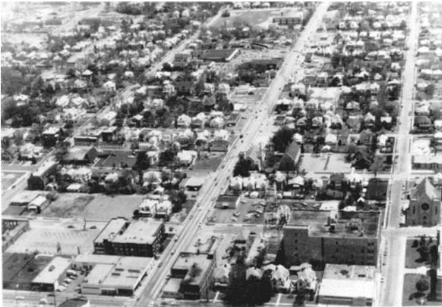
Figure 2-1. Typical terrain representative of Exposure B.
