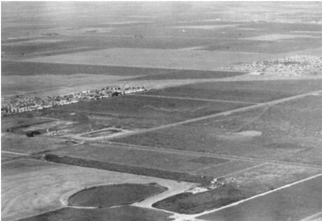
Figure 2-2. Typical terrain representative of Exposure C.
