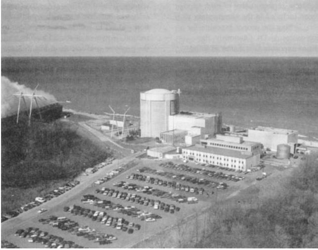
Figure 2-3. Typical terrain representative of Exposure D.
