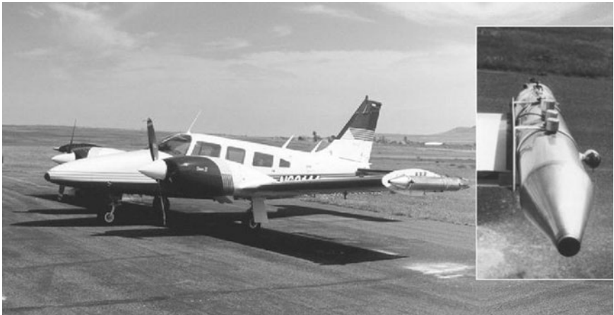
FIGURE 5-2. Acetone-Silver Iodide Generator Mounted on a Wing Tip (ASCE, 2004).
