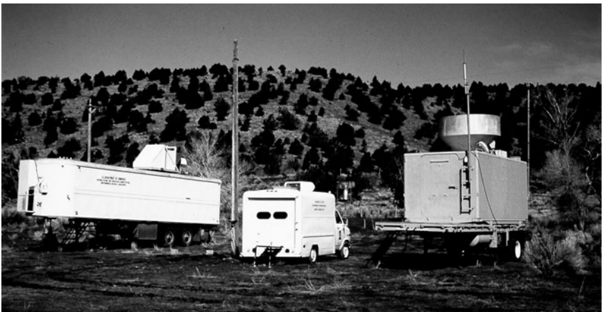
FIGURE 5-14. Microwave Radiometer, left, and Lidar, center (Griffith et al., 1995).
