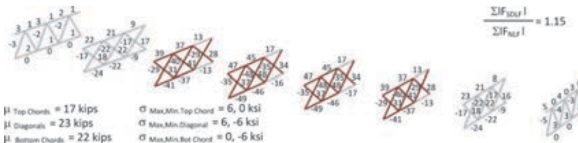
Figure 3-73. Bridge NISCR2 maximum amplitude of the component axial forces in each of the cross-frames under total dead load, SDLF detailing of the cross-frames.
