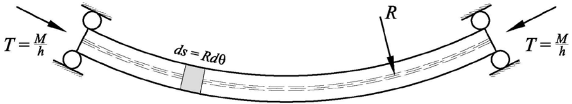
(a) Axial forces in the top flange due to uniform moment
