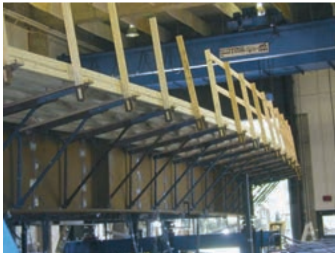
Figure 3-5. FHWA Test Bridge, overhang brackets attached to the fascia girder on the outside of the curve (Girder G1 per the NCHRP Project 12-79 naming convention, Girder G3 in reports and papers on the FHWA research) (Jung, 2006; Jung and White, 2008).
