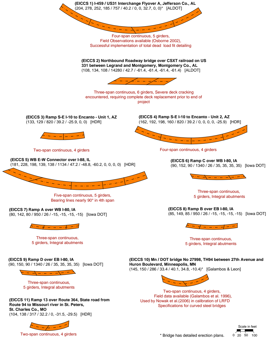
Figure 4.6. Existing I-girder bridges, Continuous-span, Curved with Skewed supports, (EICCS #) Description (LENGTH1, LENGTH2, ... / RADIUS / WIDTH / \theta_{Left} , ..., \theta_{Right} ) [Source].
