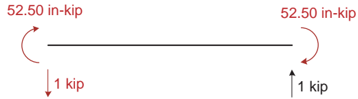
Figure 3-16. Cross-frame nodal shears and moments and equivalent Euler-Bernoulli beam shears and moments based on shear analogy.
