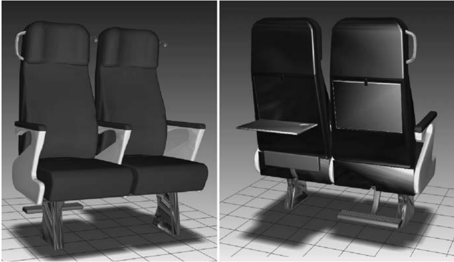
Fig. 2.4 Concept 4 for the style today ( armrests : fixed; lighting : lateral; footrest : yes; table : yes)
