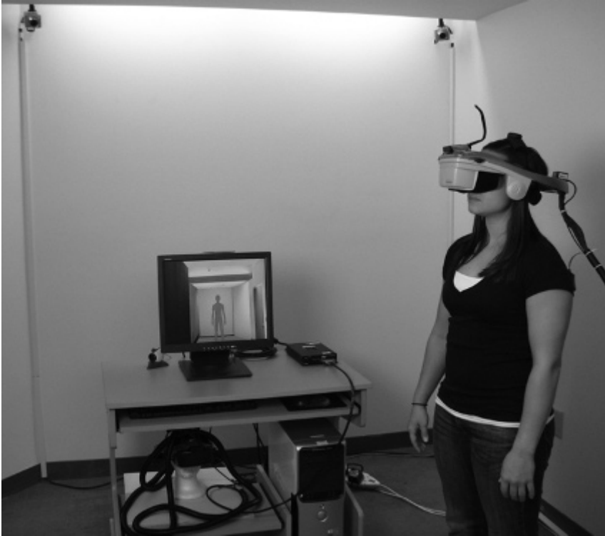
Figure 6.1 An immersive virtual environment (cameras at the corners of the room track the participant's movements to render the virtual environment appropriately in the head-mounted display she is wearing)
