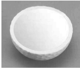
Figure 7-1. The cross-section of a two-piece golf ball (Photo courtesy of UMX Inc., www.umei.com .)
