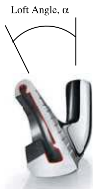
Figure 7-2. The loft is the angle the club face makes with the vertical.
