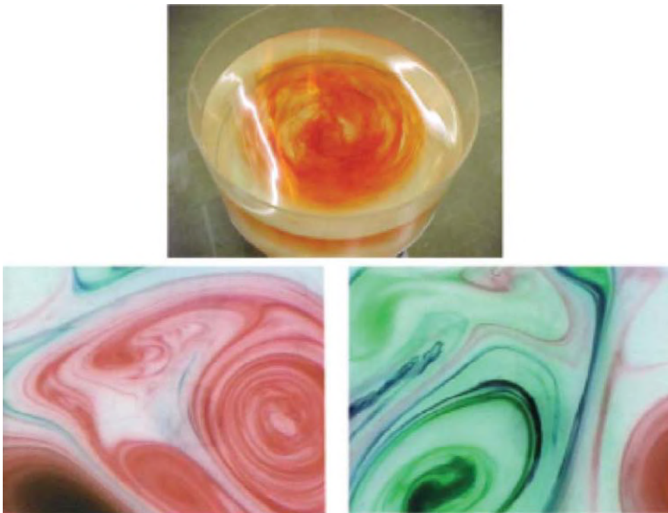
FIGURE 6. Taylor columns revealed by food coloring in the rotating tank. The water is allowed to come into solid body rotation and then gently stirred by hand. Dyes are used to visualize the flow. At the top we show the rotating cylinder of water with curtains of dye falling down from the surface. Below we show the beautiful patterns of dyes of different colors being stirred around one another by the rotationally constrained motion.
