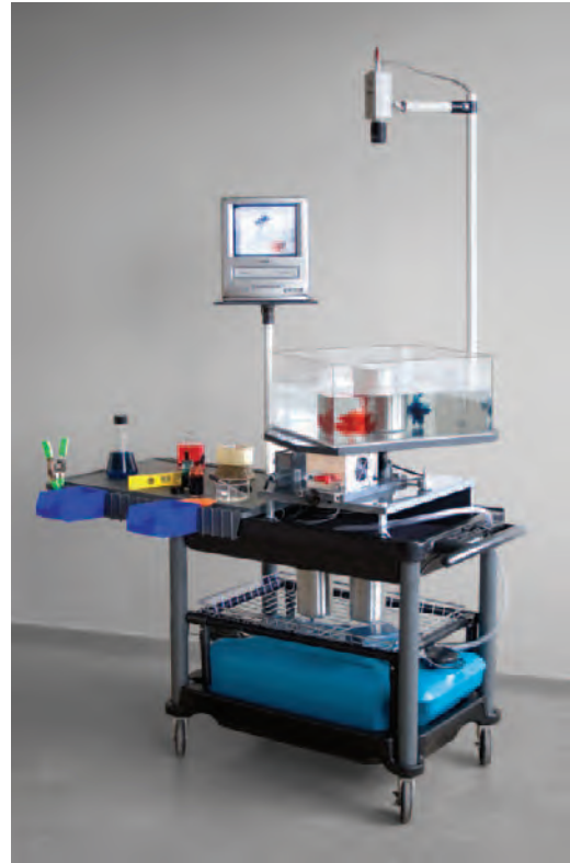
FIGURE A.1. A turntable on a mobile cart equipped with a water storage tank and pump, power supply, and monitor. A tank filled with water can be seen with an ice bucket in the middle, seated on the turntable, and viewed through a co-rotating overhead camera.
