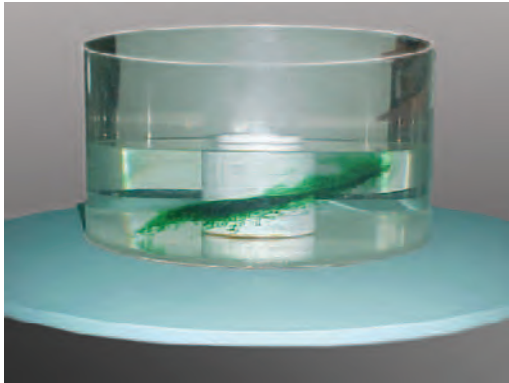
FIGURE 7.13. Dye streaks being tilted over into a corkscrew pattern by an azimuthal current in thermal wind balance, with a radial temperature gradient maintained by the ice bucket at the center.
