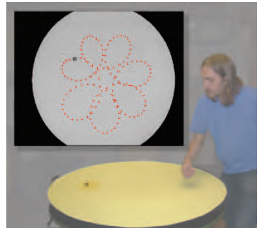
FIGURE 6.13. Studying the trajectories of ball bearings on a rotating parabola as described in Durran and Domonkos (1996). A co-rotating camera views and records the scene from above.
