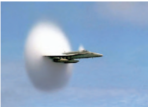
FIGURE 1.8. A photograph of the sound barrier being broken by a US Navy jet as it crosses the Pacific Ocean at the speed of sound just 75 feet above the ocean. Condensation of water is caused by the rapid expansion and subsequent adiabatic cooling of air parcels induced by the shock (expansion/compression) waves caused by the plane outrunning the sound waves in front of it. Photograph was taken by John Gay from the top of an aircraft carrier. The photo won First Prize in the science and technology division of the World Press Photo 2000 contest.
