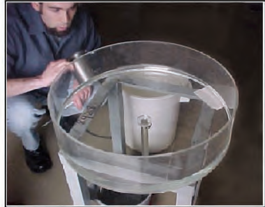
FIGURE 6.20. A leveled cylinder is filled with water, covered by a lid and left standing for several days. Attached to the small hole at the center of the cylinder is a hose (also filled with water and stopped by a rubber bung) which hangs down in to a pail of water. On releasing the bung the water flows out and, according to theory, should acquire a spin which has the same sense as that of the Earth.
