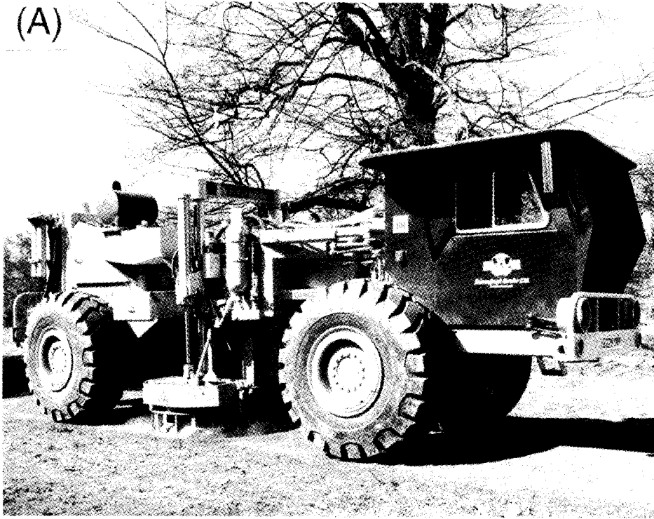
Figure 4.28 (A) A Vibroseis truck. The weight of the vehicle is transferred to the jack in the middle of the vehicle when operating (Courtesy of SSL) (B) Schematic of a Vibroseis truck. Courtesy of BP
