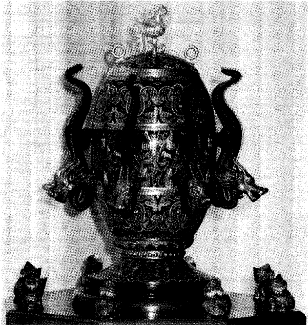
Figure 4.39 The earliest known seismoscope was developed in 132 by Heng Zhang and was used successfully to indicate the occurrence of an earthquake in the year 138. Courtesy of Stop Disasters and the World Intellectual Property Organization
