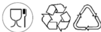
Fig. 53.5 Symbols of food-contacting and recyclable packaging to be used in food labeling, according to the TR TS 005/2011 technical regulation
