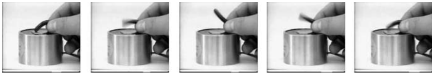
Fig. 28 Snapshot of shape change of a magnetoelast due to modulated magnetic field. The frequency of the field is 40 Hz
