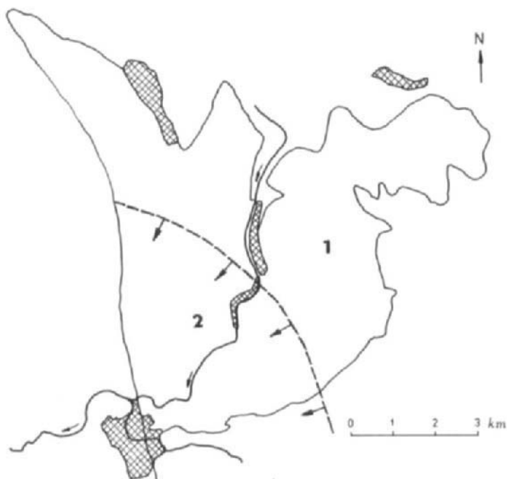
5.7 Region consisting of area suitable for groundwater recharge – 1, and impervious formations – 2 under which an artesian groundwater storage is formed.
