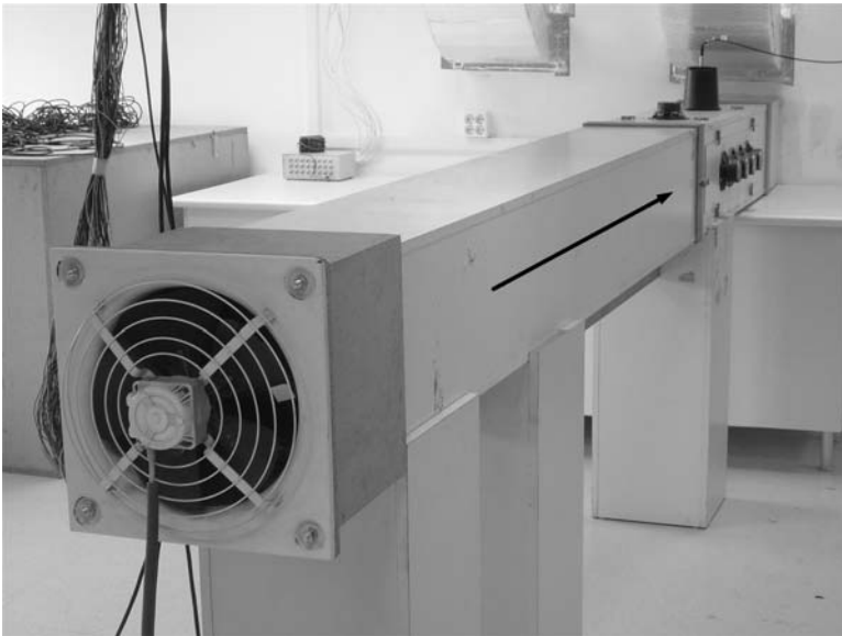
Fig. 8.13. Tube and input noise source (fan)
