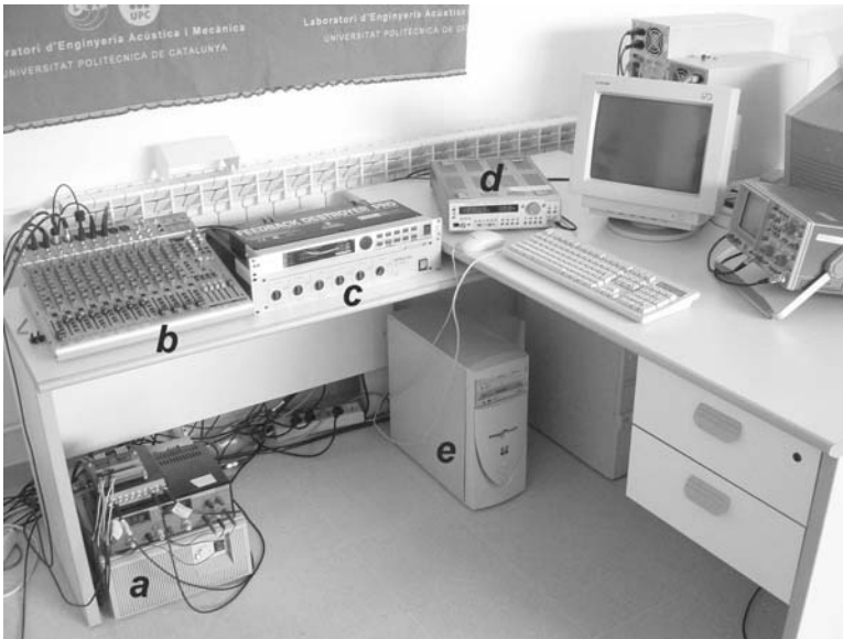
Fig. 8.15. Signal-processing instrumentation composed by (a) DSpace system, (b) mixing console, (c) audio amplifier, (d) signal generator, (e) host PC, plus the oscilloscope
