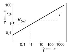
**Figure 4.19.** Constructing a log–log plot of an Ostwald–De-Waele flow behavior curve
