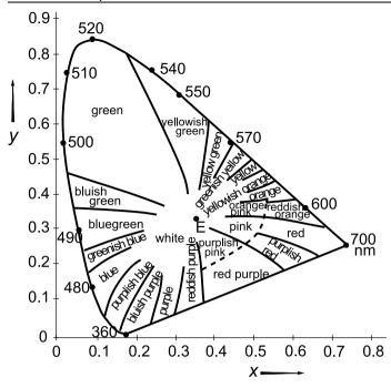
**Figure 11.4.** Chromaticity diagram. In the triangle are all colors which can be observed. Colors with maximum brilliance are on the horse shoe curve. Point E in the middle is zero brilliance (white)
