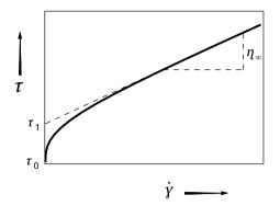
Figure 4.20. Determining the extrapolated yield stress  $\tau_1$  for the WINDHAB model
