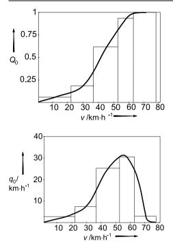
Figure 15.1. Sum distribution curve showing accumulation of sum fraction of speed measurements in velocity class categories as a function of velocity
