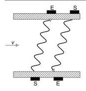
Figure 14.4. Ultrasonic flow meter. The run time of a pulse from sender S to receiver E is shorter in the direction of the flow than in the opposite direction
