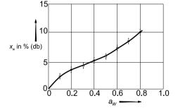
Figure 1.15. Sorption isotherm of microcrystalline cellulose (25 °C, adsorption) (from [23])
