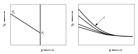
Temperature gradient is constant over time perature gradient is a function of time
