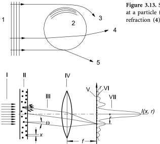
**Figure 3.13.** Scattering of light (1) at a particle (2) by diffraction (3), refraction (4) and reflection (5)
