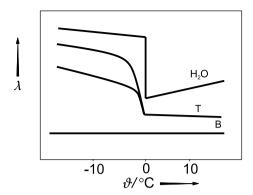
**Figure 7.11.** Thermal conductivity of water (H<sub>2</sub>O), butter (B) and turkey meat (T). T: upper curve indicates  $\lambda$  parallel to fiber, lower curve  $\lambda$  perpendicular to meat fiber [115]
