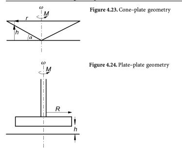
for highly viscous materials (emulsion, paste, whipped cream) which would otherwise not flow easily into the narrow cylindrical annular space of a coaxial rotational rheometer. The plate-and-plate rheometer is particularly useful for suspensions that have relatively large particles (e.g. 50 microns) such that a cone-and-plate would be too narrow for them.
