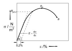
**Figure 4.4.** Stress-strain diagram of a material with a smooth profile showing no distinct yield point.  $R_{p0.2}$  is the technical limit of elasticity for the 0.2 strain limit technique. The slope of the straight line portion gives the modulus of elasticity *E* for the material. The highest point on the curve ( $R_m$ ) gives the maximum strength of the material. *B* is the rupture point (rupture strength)
