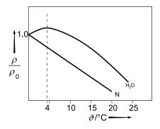
**Figure 2.3.** Abnormality of water  $(H_2O)$ : Temperature dependency of density compared to normal behavior (N)
