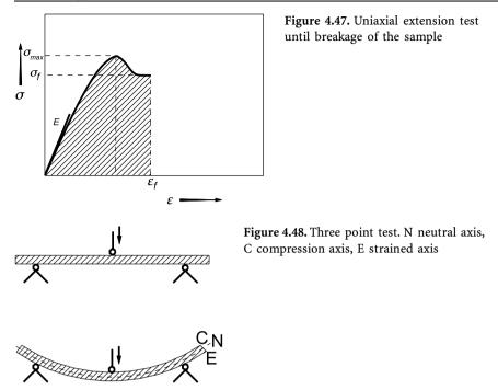
consumer. In order to conduct such tests with samples of such unique configuration and geometry, a host of specialized sample holders may be needed, such as shown in Figure 4.48 [12] for samples which are long (large length to width ratio).
