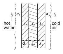
**Figure 7.10.** Multilayer heat transfer with convection on both sides. Example: Material 2 is steel, 1 is rust and 3 is paint. The overall heat transfer coefficient k is given in equation (7.102) below.
