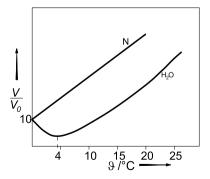
**Figure 2.2.** Normal (N) and abnormal (H<sub>2</sub>0) thermal expansion (schematic)
