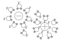
Figure 8.6. Ions with surrounding water molecules – hydrated ions
