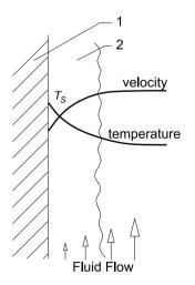
Figure 7.9. Convection heat transfer. Showing boundary layer where velocity and temperature profiles exist near wall surface, 1: hot wall, 2: boundary layer region of bulk fluid flow is reached, where the fluid velocity is all the same at the maximum. This region is known as a boundary layer.
