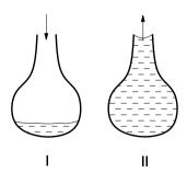
**Figure 1.3.** The capillary radius on adsorption (I) is different from that on desorption (II) when a pore has the shape of a bottle or flask (schematic)
