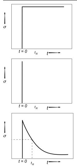
Figure 4.33. Stress response to a sudden constant deformation. Ideal elastic sample (upper picture), ideal viscous sample (middle) and viscoelastic sample (shown at the bottom).
