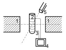
Figure 9.9. Schematic of an NMR spectrometer. 1: magnet, 2: sample holder, 3: receiver coil, 4: computer, 5: radio wave transmitter
