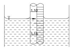
Figure 2.9. Hydrometer. 1: scale, 2: body (with and without thermometer), 3: keel
