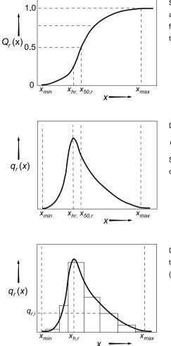
Summation distribution function showing accumulation of "pass through" fraction as a function of sieve size ("accumulating pass through diagram")
