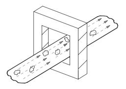
**Figure 14.3.** Tunnel-type metal detector with food product on a conveyer belt (schematic)
