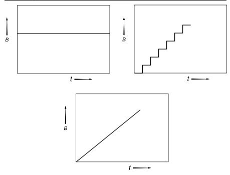
**Figure 4.49.** Types of tests: Static (upper left diagram) and dynamic (lower diagram) loading of a sample. The stepwise test is in the upper right middle diagram.
