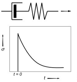
Figure 4.34. MAXWELL model element: spring and dashpot in series.
