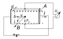
Figure 9.4. HALL sensing probe for measuring magnetic field strength (schematic)
