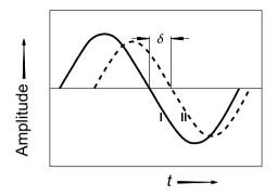
**Figure 4.42.** Phase shift between deformation  $\gamma$  (I) and shear stress  $\tau$  (II)
