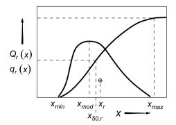
**Figure 3.11.** Median value  $x_{50,r}$ , modal value  $x_{mod}$  and average  $x_r$  (integral mean) of the  $q_r(x)$  curve [1]
