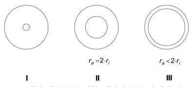
Figure 7.7. Thick walled tube (I) and thin walled tube (III). II is borderline between I and III
