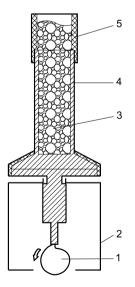
Figure 2.15. Device for tapping of bulk goods: 1: rotating cam, 2: housing, 3: powder sample, 4: cylinder, 5: overring
