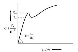
**Figure 4.3.** Stress-strain diagram of a material with a distinct yield stress  $R_{eH}$
