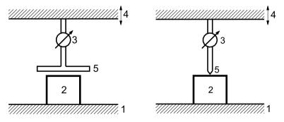
Figure 4.50. Compression test between parallel plates (left). Penetration test or cutting test (right). 1: platform or workbench,, 2: sample, 3: load cell (force meter), 4: movable crosshead, 5: individual testing tool
