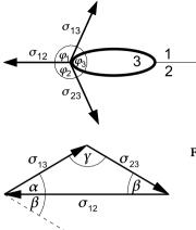
Figure 5.8. Interfacial tensions at the point where three phases are in contact. For example, phase1 is a gas, phase 2 is liquid A, and phase 3 is liquid B.
