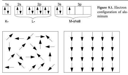
**Figure 9.2.** Aluminum without outer magnetic field (left). aluminum in an outer magnetic field is magnetically polarized (right)
