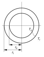
Figure 7.6. Temperature profile across a single-layer cylindrical wall
