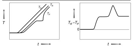
**Figure 7.29.**  $\Delta T = T_r - T_P$  versus time during a DSC run
