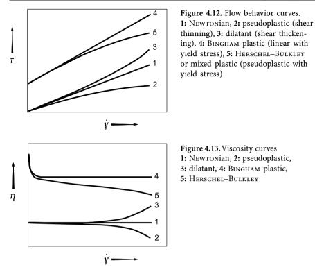
stress-shear rate diagram, we call this non-NEWTONian flow behavior. The flow behavior of non-NEWTONian fluids depends on the stress conditions to which the fluids are subjected. Some typical flow behavior curves are summarized in Figure 4.12.
