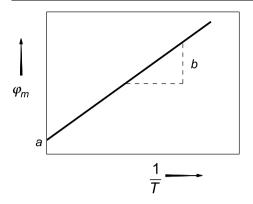
Figure 10.1. Temperature dependency of polarization potential
