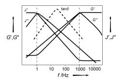
**Figure 4.43.** Oscillation testing of a viscoelastic material (schematic)
