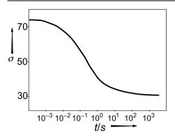
Figure 5.20. Tension versus surface age (schematic)
