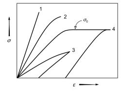
**Figure 4.53.** Stress strain curves: 1: ideal elastic, 2: nonlinear elastic, 3: nonlinear elastic plastic, 4: plastic.  $\sigma_0$  is the yield stress
