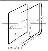
Figure 8.7. Partly filled plate capacitor
