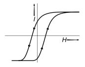
Figure 9.3. Hysteresis behavior in a ferromagnetic material
