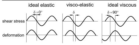
Figure 4.41. Phase shift during an oscillating shear load
