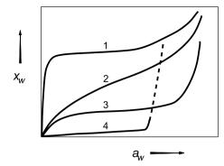
Figure 1.6. Examples of water vapor sorption isotherms. 1: silica (strong sorbent), 2: milk powder (multilayer forming material), 3: black tea (monolayer forming material), 4: fructose (nearly impervious to water, then rapid uptake of water until a syrup is formed)
