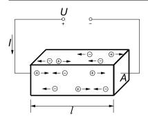
Figure 8.1. Food with electric current passing through (schematic)
