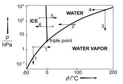
Figure 15.8. Phase diagram of water
