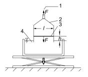
Figure 5.13. Schematic for measuring surface tension with the bow wire. 1: forcemeter, 2: bow wire, 3: horizontal piece of wire, 4: liquid sample
