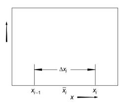
**Figure 3.8.** Particle sizing: Definition of a category *i*, arithmetic mean  $\overline{x_i}$ and an interval width  $\Delta x_i$
