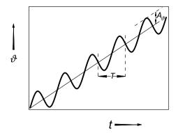
Figure 7.39. Temperature modulated heating rate
