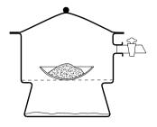
**Figure 1.14.** Taking a point of the sorption isotherm. The sample is placed in a closed chamber with a humidity standard (at the bottom, schematic). After water activity equilibration of sample and atmosphere in the chamber the sample is weighed to get its moisture content
