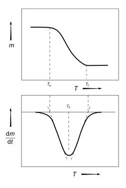
**Figure 7.24.** TG and DTG signal curves. Beginning  $T_e$  and end  $T_f$  of the transition can be read out as extrapolated temperatures.  $T_p$  is the peak temperature, it is the temperature where the mass flux has its maximum [15]
