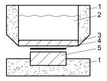
**Figure 7.19.** FITCH apparatus for measuring thermal conductivity [134]. 1: insulation, 2: liquid with temperature T<sub>S</sub>, 3: and 5: copper block, 4: sample
