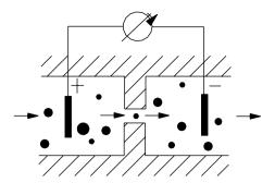
**Figure 3.15.** Electrical counting of particles with different sizes through a capillary tube (schematic)
