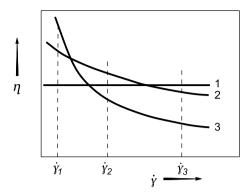
Figure 4.14. NEWTONIAN fluid (1), and non-NEWTONIAN fluids (2,3) in comparison
