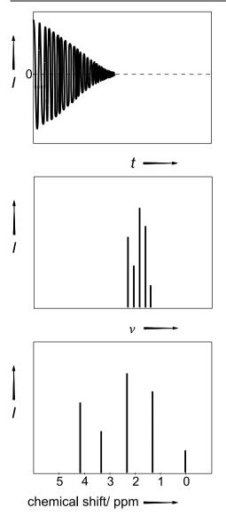
**Figure 9.11.** HR-NMR: By FOURIER transformation of the free induction decay (upper picture) we get the intensities of the resonance frequencies (picture in the middle) of a sample. Often the frequency shift related to a standard is used is such spectra (picture at the bottom)
