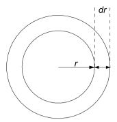
Figure 5.3. Volume increase of a liquid droplet (needs energy because of surface tension)
