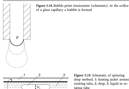
Figure 5.19. Schematic of spinning drop method. 1: heating jacket around rotating tube, 2: drop, 3: liquid in rotating tube
