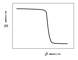
Figure 7.27. TG calibration with a nickel standard. On reaching the CURIE temperature (for nickel  $351.4 \pm 4.8$  °C) the magnetic attraction disappears and the mass signal shows a sudden decrease.
