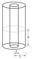
The last equation shows that the capacitance is a linear function of the filling height *h*. So, we have a filling height monitor. When a cylindrical capacitor like the one shown in Figure 8.9 is used, we have:
