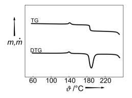
**Figure 7.26.** TG of aspartame. Note the mass drop on heating above baking temperatures of 180 °C.
