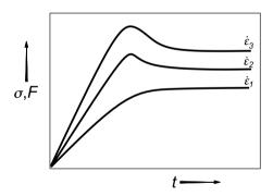
**Figure 4.44.** Flow test with a viscoelastic material. After reaching the yield stress at a constant rate of axial deformation or strain  $\dot{\epsilon}$  the sample shows a constant stress indicating flow. Measuring the force *F* instead of a stress  $\sigma$  give a similar diagram.
