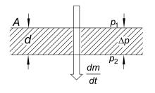
**Figure 6.3.** Permeation through a film (schematic)
