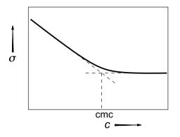
Figure 5.5. Surface tension as function of emulsifier concentration
