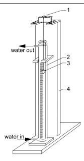
**Figure 2.12.** Floating technique. The sample P is suspended in the fluid F
