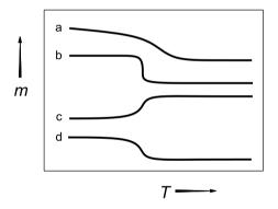
**Figure 7.23.** TG signals (schematic): (a) evaporation, drying, sublimation; (b) boiling in pan with small hole; (c) sample oxidation; (d) CURIE transition
