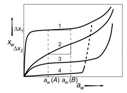
**Figure 1.9.** Exposing four materials exhibiting different degrees of hygroscopicity to a shift in water activity from  $a_W(A)$  to  $a_W(B)$ . The same shift causes different amounts of water uptake  $\Delta x$
