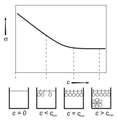
**Figure 5.6.** After reaching the monolayer at the critical concentration point, cmc, the surface tension remains constant with increasing concentration.
