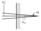
**Figure 7.20.** Heat probe sensor to measure thermal conductivity (after SWEAT et al [5]), showing needle-type heating element H with electrical voltage potential ( $U_H$ ) for power to heat source, and voltage potential from thermocouple junction ( $U_{Th}$ ) for temperature measurement
