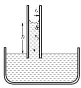
**Figure 5.15.** Capillary action (rise in liquid level in capillary tube) to evaluate interfacial tension
