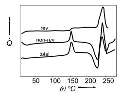
**Figure 7.40.** MDSC plot of a semicrystalline carbohydrate. The glass transition can be seen in the reversing signal (rev). The classic DSC signal (total) does not show the glass transition because it is hidden by another thermal event [24]
