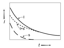
**Figure 9.12.** Solid (s) and liquid phase (l) show different relaxation behavior. The measured FID (1 + s) is the result of addition of both parts
