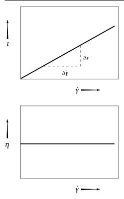
**Figure 4.11.** Flow behavior curve (upper diagram) and viscosity curve (lower diagram) of a NEWTONIAN fluid. The slope  $\eta$  of the upper curve is constant for all shear rates.
