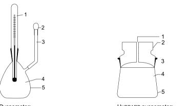
Pycnometer: 1 thermometer, 2 cap, 3 capillary, 4 sample, 5 glass bulb HUBBARD pycnometer: 1 capillary, 2 glass stopper, 3 wide opening, 4 sample, 5 glass bulb
