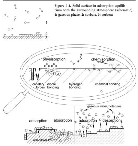
Figure 1.2. Types of binding and terms used in sorption
