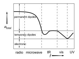
**Figure 10.2.** Frequency dependency of the electric polarization potential [113]
