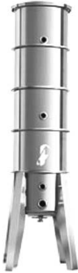
Fig. 18.4 A spinning-cone column apparatus [22]
