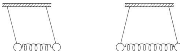
Fig. 10.9. The fundamental oscillations of two coupled pendulums: symmetric and antisymmetric oscillations (normal modes)
