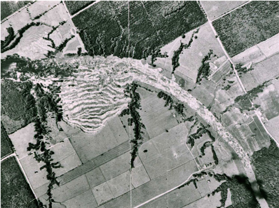
Fig. 9.8 The 1971 South Nation River landslide. This rapid spread was contained laterally, by pre-failure gullies (Canada Airphoto A30362: 152)
