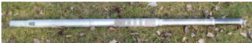
Fig. 17.1 The CPT-R probe used in this study. CPT, resistivity and battery modules comprise a probe with a total length of 1,125 mm
