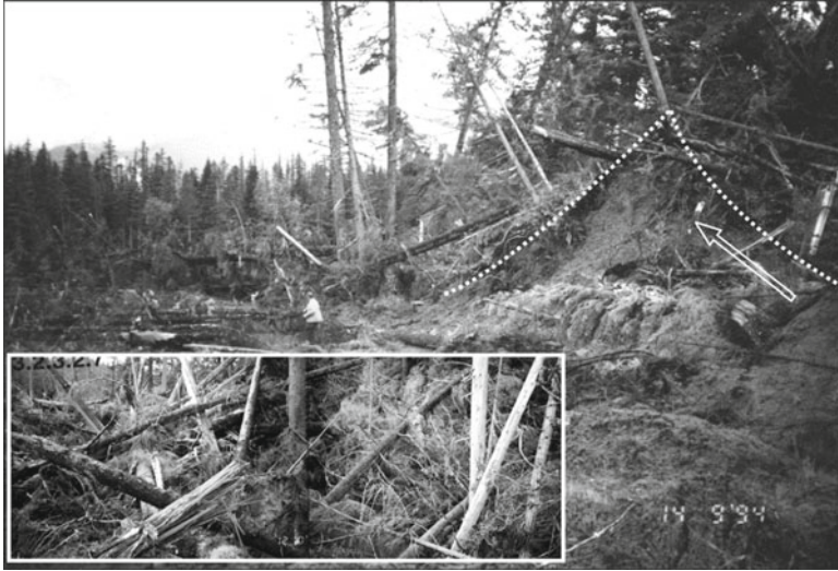
Fig. 9.5 Interlocking networks of large trees add cohesion to the displaced mass (locally) at the Mink Creek landslide (Note how the displaced material has piled up against trees ( arrow ))
