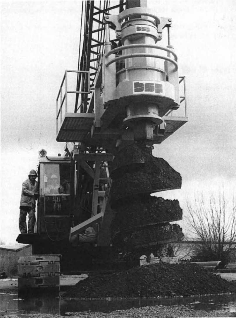
Figure 6.27 Crane mounted earth auger capable of boring a 2 m diameter hole to about 44 m depth. Larger and deeper holes can be obtained by modifying the rig. Similar rigs can be wagon mounted. (Courtesy BSP International Foundations Ltd)
