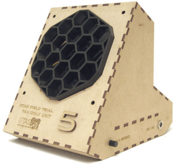
Fig. 13.22 Completed fan-only prototype
