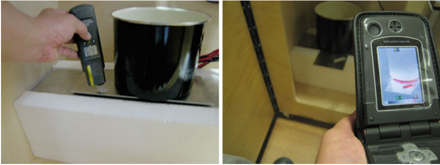
Fig. 13.69 An enamel container was used to melt the PCM. To enable a reading of T-hot, a 3 mm aluminium plate was used with a contactless thermometer reading the infrared emission off a piece of masking tape
