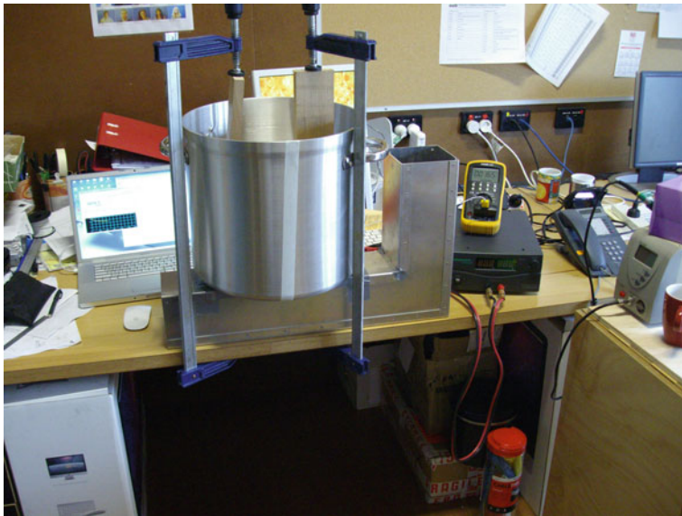
Fig. 13.75 Engineered stockpot being clamped to cooling fin assembly in duct
