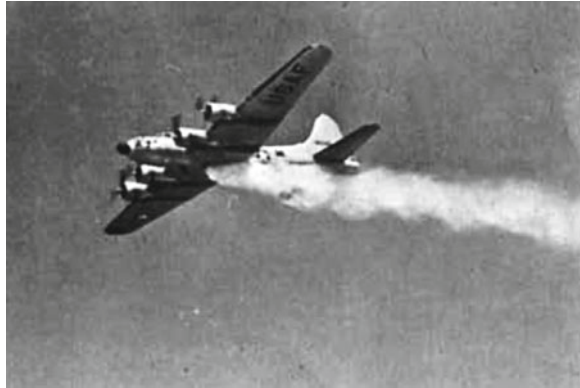
Fig. 7.2 Cloud seeding using a water spray from a B-17 airplane used by the University of Chicago. Image credit Battan (2003)
