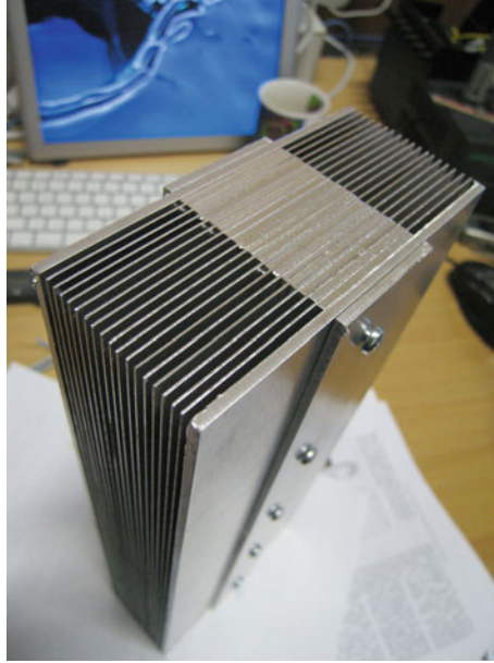
Fig. 13.48 Cooling fins assembled with bolts
