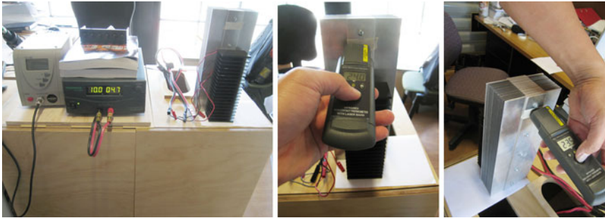
Fig. 13.49 Setup to test efficacy of heat transfer through the spacers of the cooling fin
