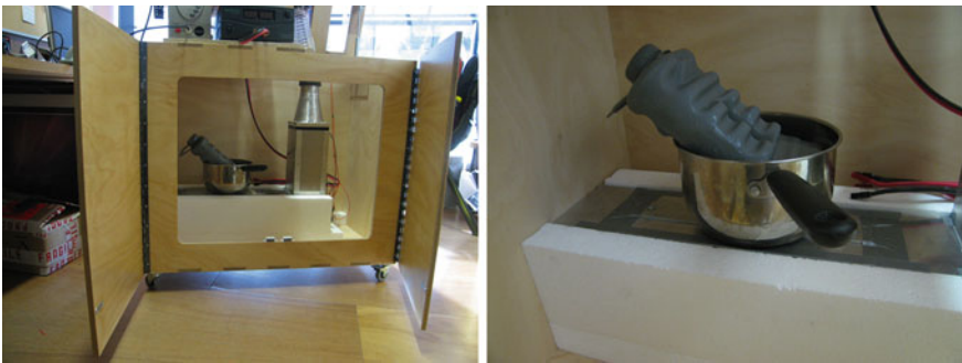
Fig. 13.70 Stainless steel saucepan holding a water and a frozen bottle to simulate the refrigeration from TE modules
