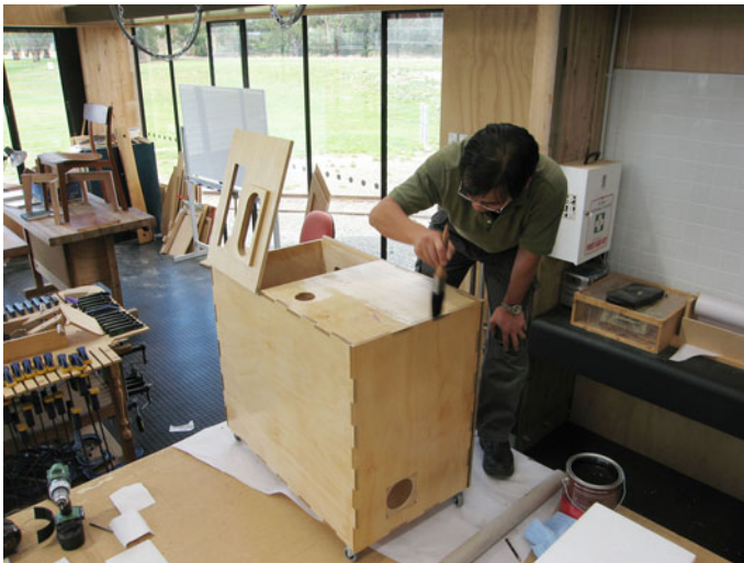
Fig. 13.40 Application of polyurethane varnish
