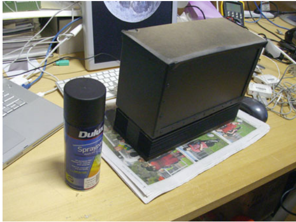
Fig. 13.65 Tank and fins coated with 2 layers of matte black spray paint
