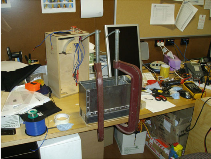
Fig. 13.9 Use of clamps to minimise TIM thickness was effective and routinely adopted in future prototypes
