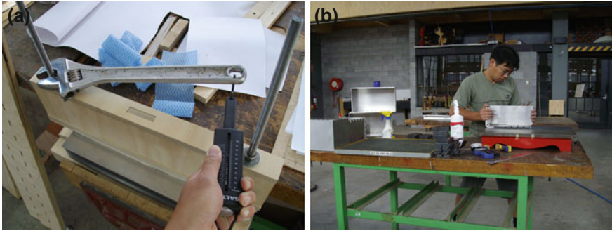
Fig. 13.16 To ensure consistency, a the torque applied to the nuts was measured, and b weights applied, number of strokes and angle of strokes in sanding were kept consistent
