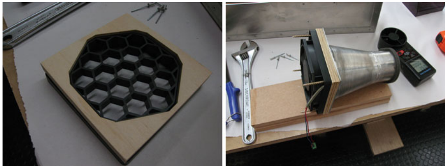
Fig. 13.25 Honeycomb and spacers to create a flushed face on which to bolt the funnel
