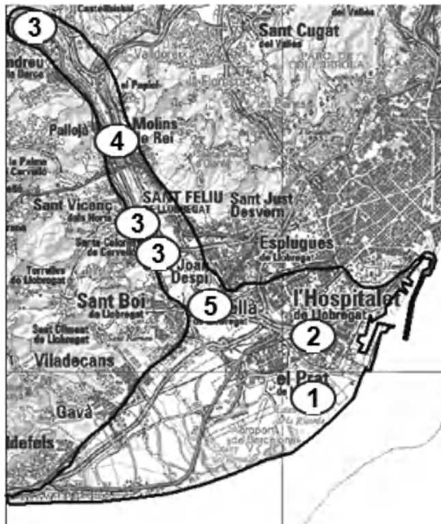
Figure 17.3 Activities to improve water quantity and quality in the Llobregat's lower valley and delta aquifers: 1 – wastewater treatment plant, 2 – injection barrier to control seawater intrusion, 3 – recharge ponds, 4 – riverbed scarification, 5 – well injection.
