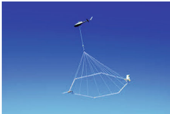
Fig. 4.25 HeliTEM survey operation with transmitter and receivers
