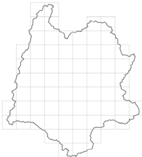
Figure 6. Discretization of model domain into a finite difference grid.
