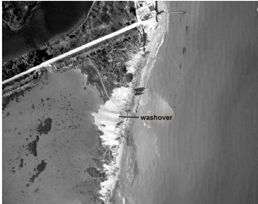
Figure 6. Example of seawater inundation caused by a winter storm and formation of washover fan (Vene Ancona-Bellocchio in 2005)
