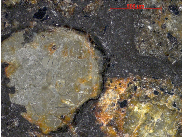
Fig. 2.4 A thin section of GRA95229 from the NASA Antarctic collection that shows several silicate chondrules and the dark fine-grained matrix compacting the structure (J.M.Trigo/CSIC-IEEC)
