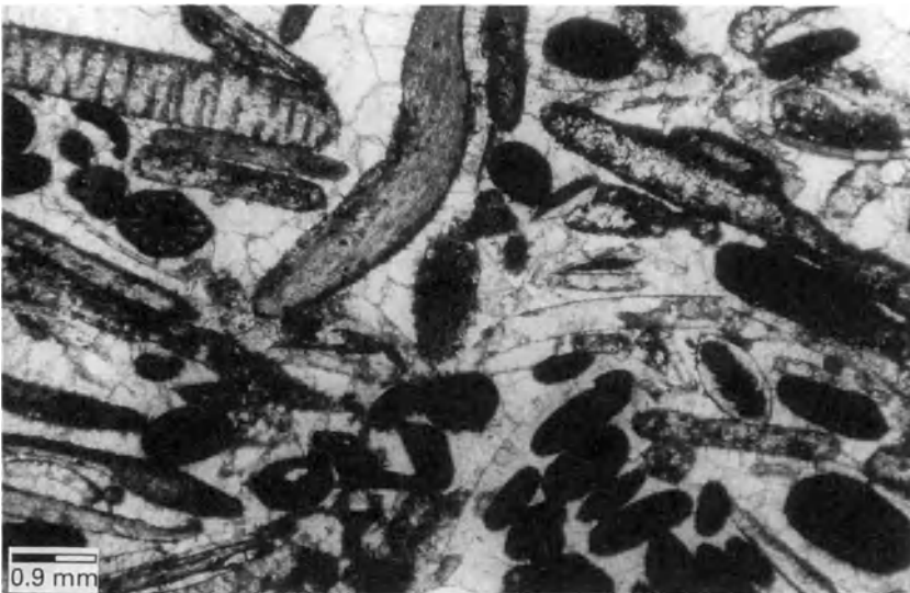
Figure 10.4 Calcareous limonite oolite, Lias, central England. Dense limonite ooids and peloids intermingled with abraded shell debris and set in a sparite cement. A low-quality ore body. Polarized light.
