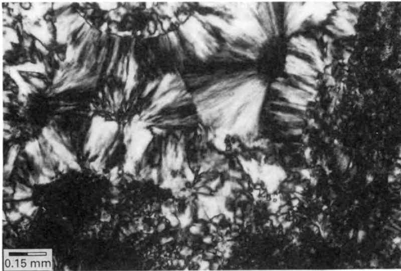
Figure 9.7 Enlargement of Figure 9.6 to show the detail of the radiating fibrous chalcedony. Crossed polars.
