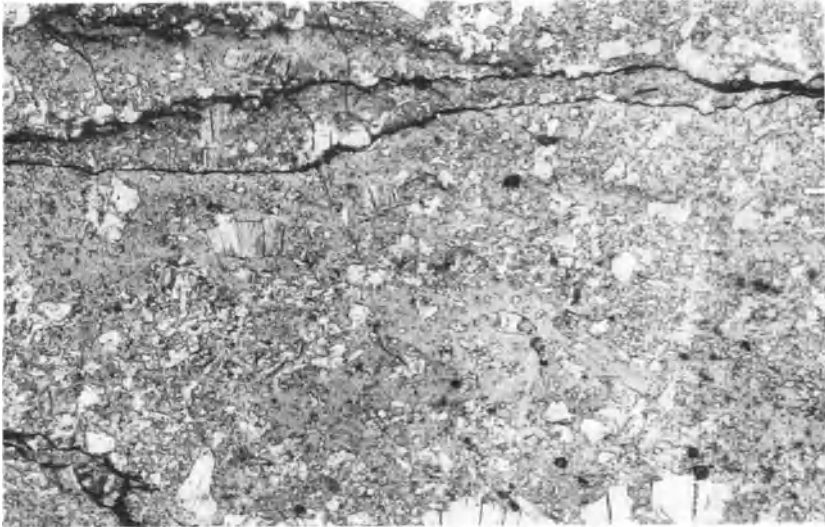
Figure 14.7 Tonstein, Coal Measures, northern England. Laths and vermicules of clear kaolinite set in a pale brown matrix of cryptocrystalline kaolinite. Carbonaceous (coal) films are common. Polarized light. Scale bar = 0.9mm.
