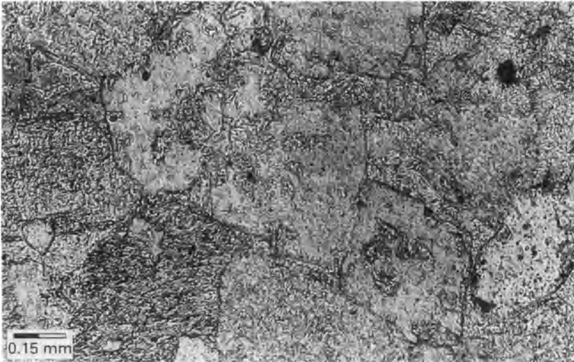
Figure 8.4 Dolomite, Permian, northern England. A sucrose or saccharoidal dolomite with a dense intergrowth of dolomite grains mostly showing a good euhedral rhombic shape. This texture is also known as idiotopic. Polarized light.
