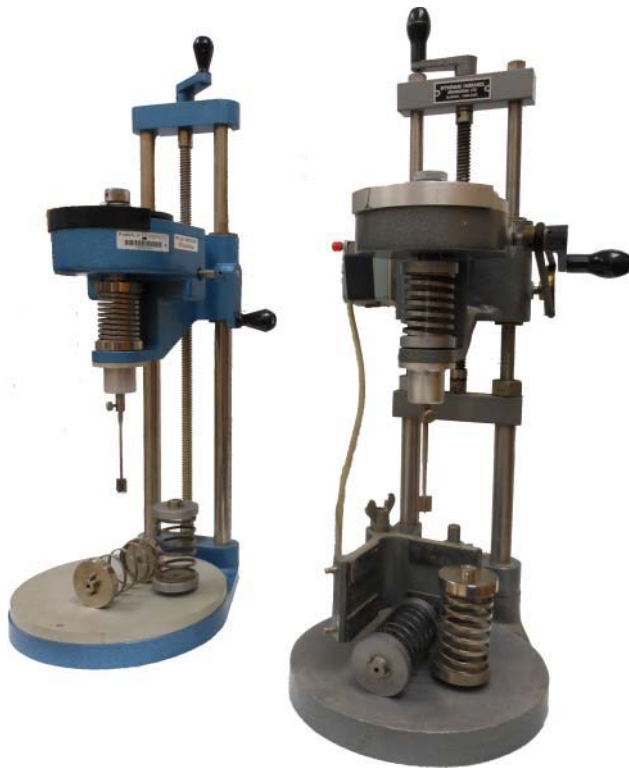
Figure 5.29 Miniature vane shear apparatuses showing set of calibrated torque springs.
