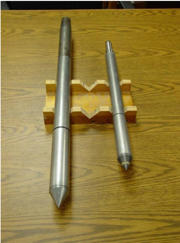
Figure 5.12 Cone penetrometers: 15 cm 2 cone on the left and 10 cm 2 cone on the right.
