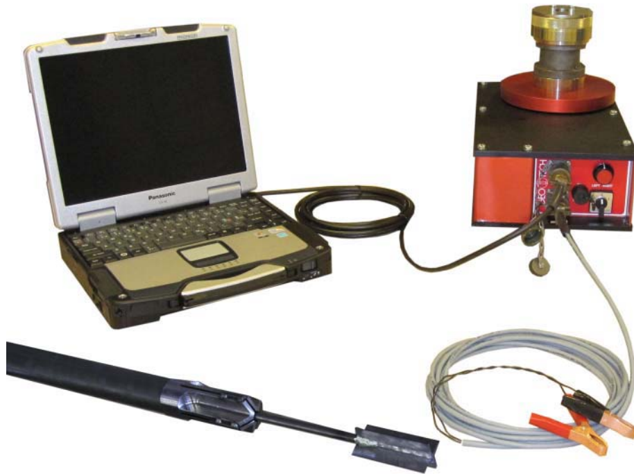
Figure 5.35 Direct-push vane shear apparatus with electronic drive unit. Photo courtesy of Ingenjorsfirman Geotech AB, Sweden.
