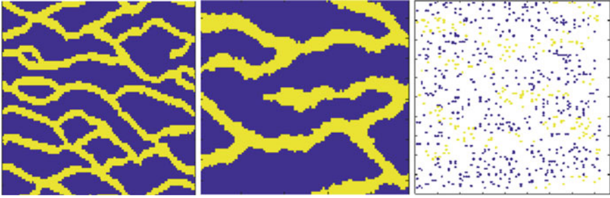
Fig. 27 The available TI ( in the left ), the corrected map with different geobody size ( in the middle ), and the scattered data sampled from the correct map ( in the right )
