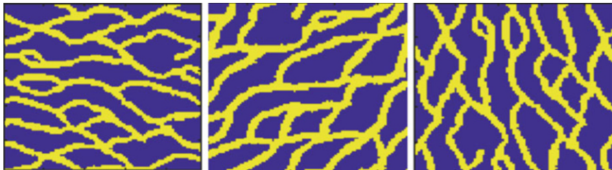
Fig. 2 Three different maps of facies type for channelized reservoirs with different orientation of channels
