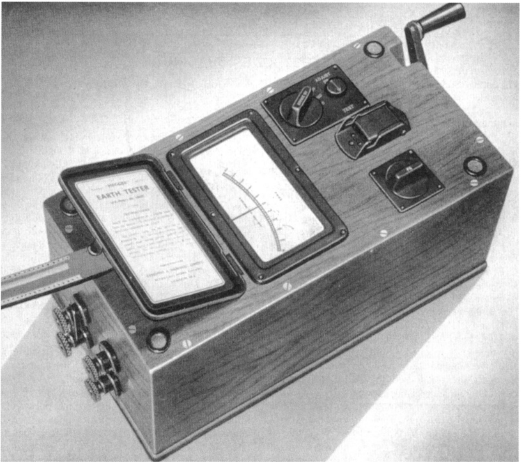
Fig. 2. The Megger Earth Tester as used by Shaw in Southern Rhodesia (from manufacturer's literature: Anon. 1950).
