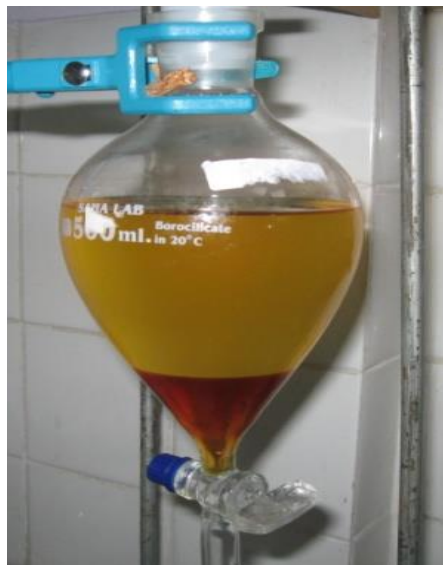
Figure 2. Corn oil biodiesel and glycerol separation (upper phase is biodiesel).
