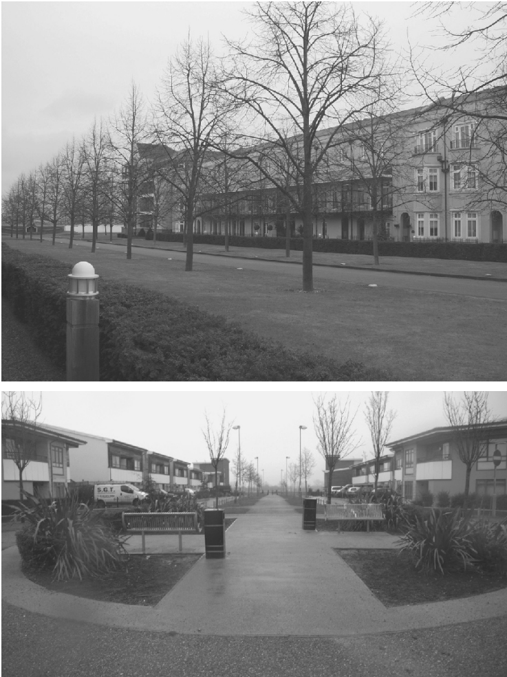
Figure 6.7 Footpaths should be located at the front of properties and be wide, well lit and direct
