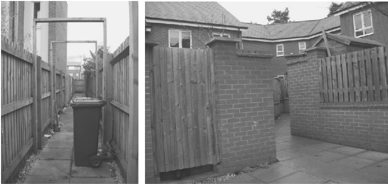
Figure 6.5 Footpaths should not run at the rear or side of properties and should be direct, well lit and overlooked
