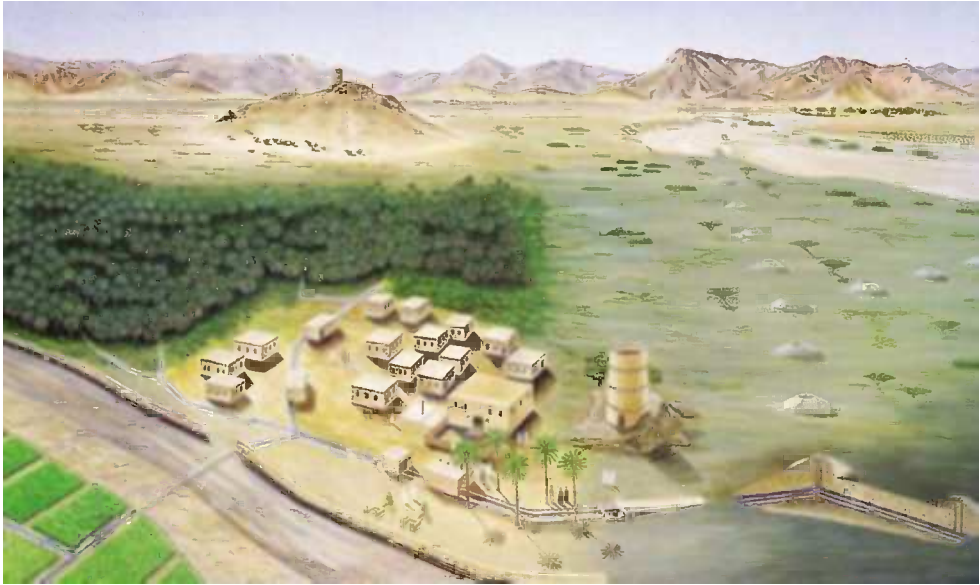
Figure 4.13 Schematic drawing of an infiltration gallery system (falaj) and its use. [Source: Oman Geologic Heritage – MRMVVR (2008)]. The main canal is excavated from the source of the falaj in mountains and wadis to cross wide areas as buried canals with holes for airing and maintenance. It discharges into open canals near the village from where it supplies irrigation ditches.
