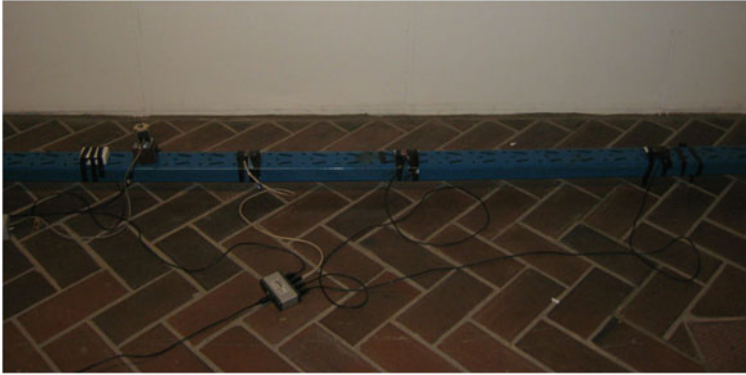
Fig. 2.3 Main section of the test beam, with wired monitoring system attached
