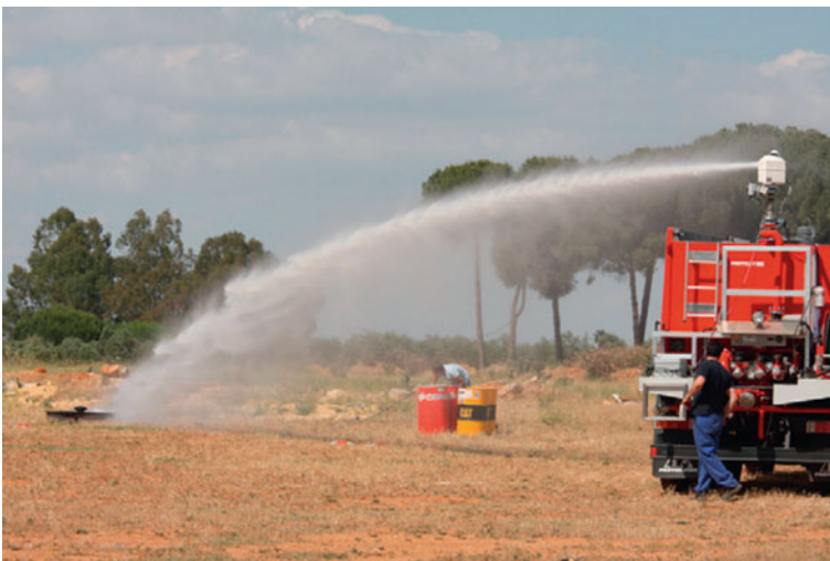
Fig. 3.13 Picture of the fire truck with the implemented fire extinguishing system
