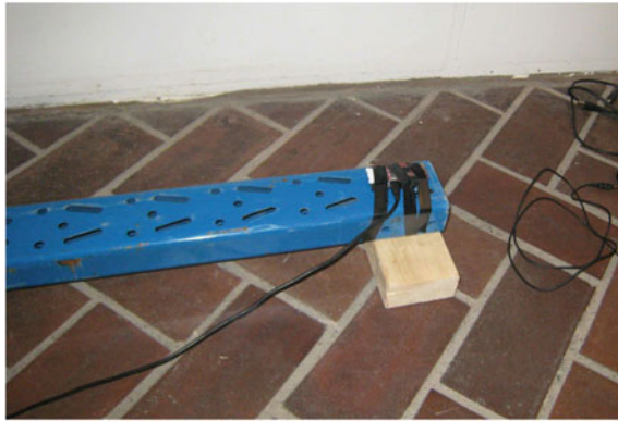
Fig. 2.3 Main section of the test beam, with wired monitoring system attached
