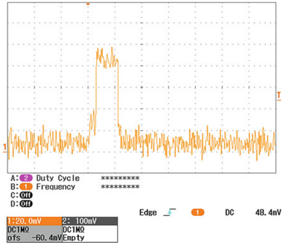
Fig. 4.5 Oscilloscope trace for an alarm packet sent to coordinator. The radio is off except when the alarm packet is sent to coordinator to signal a fall
