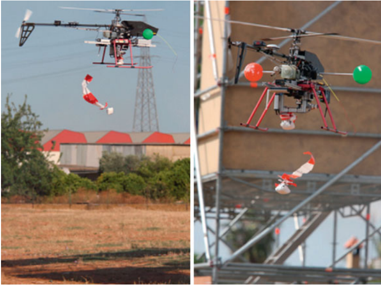
Fig. 3.12 Automatic deployment of WSN nodes using helicopters
