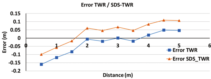
Fig. 7. Representation of SDS-TWR /TWR error as a function of the distance (Color figure online)
