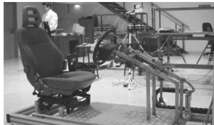
Figure 10. Vehicle seat used in the experimental setup to find the occupant initial conditions.
