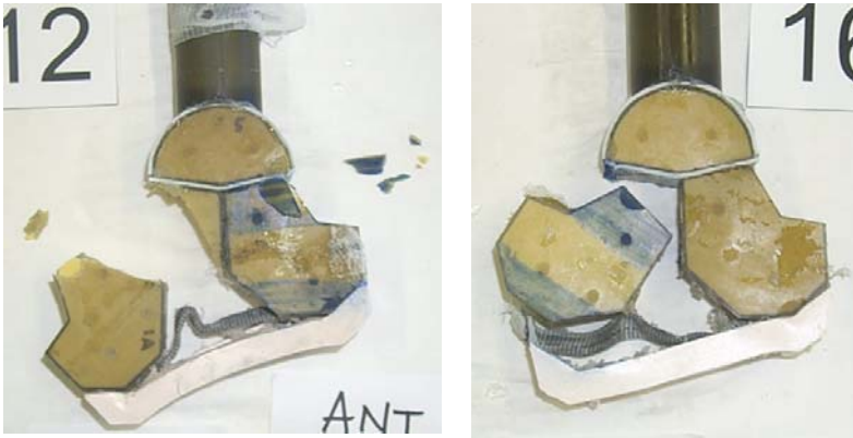
Figure 4. CLL resulting injuries for 'mine' testing without boot (left) and 'mine' testing with boot (right).
