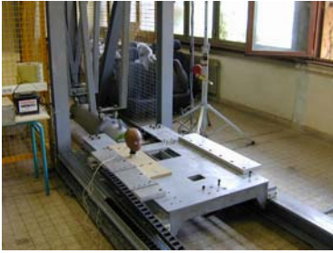
Figure 5. Q3 dummy component sled test on head and neck.
