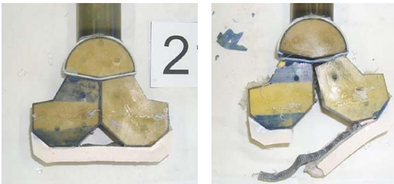
Figure 3. CLL resulting injuries for Owen-style (left) and Funk-style (right) testing.
