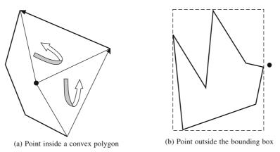
Figure 9.8 Faster point-in-polygon checks
