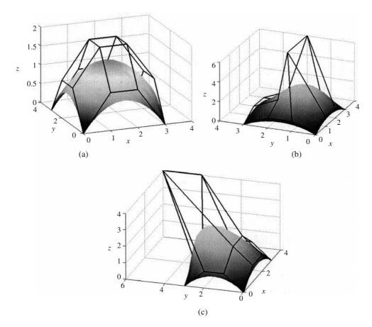
Figure 7.8 (a) Bézier bi-cubic patch in Example 7.4, (b) and (c) patches with data points relocated.
