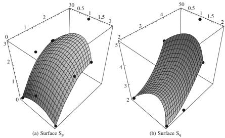
Figure 7.20 Two bi-quadratic Bézier surfaces in Example 7.10
