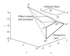
Figure 2.24 Perspective image on the x-z plane for Example 2.11
