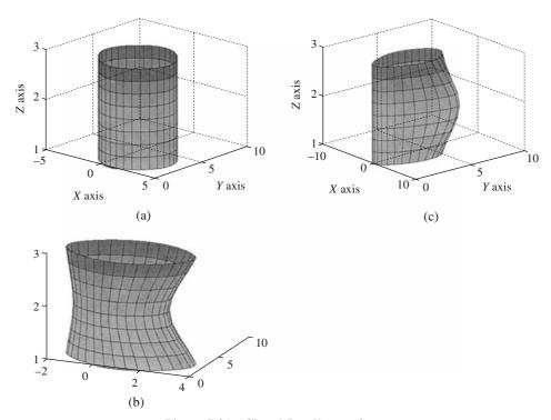
Figure 7.31 Closed B-spline surfaces
