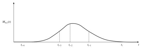
Figure 5.6 Schematic of a B-spline basis function of order 4
