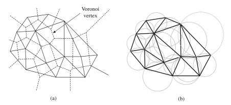
Figure A1.5 (a) Delaunary triangulation (solid) and Dirichlet tessellation (dashed) and (b) Delaunay triangles with circumcircles
