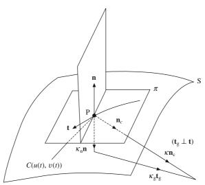
Figure 6.12 Curvature of a surface
