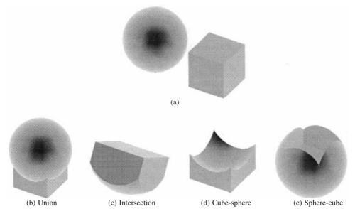
Figure 8.22 Boolean operations using a cube and a sphere
