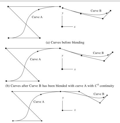
(c) Curves after Curve B has been blended with Curve A with  $C^1$  continuity
