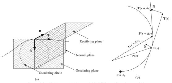
Figure 3.8  $\,$  (a) The normal plane and (b) definition of a unit normal N
