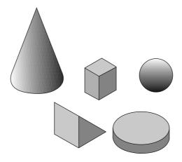
Figure 8.20 Primitive solids used in constructive solid geometry
