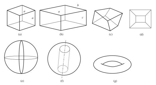
Figure 8.4 Various shapes of a hexahedral topology (a-d), all homeoporphic to a sphere in (e). A sphere with a through hole (f) is homeomorphic to a torus (g)
