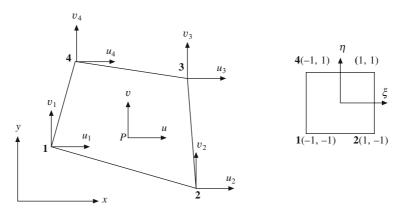
Figure 11.15 A four-node quadrilateral element
