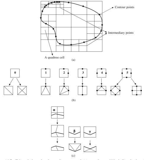
Figure A1.7 Triangulation using the quadtree approach (a) a quadtree grid including the domain such that at most one contour point lies on or within a cell (b) patterns  $0, \ldots, 5$  for cells with the intermediary points and their discretization schemes (c) internal cells intersecting with contour (dark lines) and discretization based on how the contour point is located and which region within the cell is inside the domain
