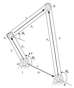
Figure 1.3 Schematic of a four-bar mechanism
