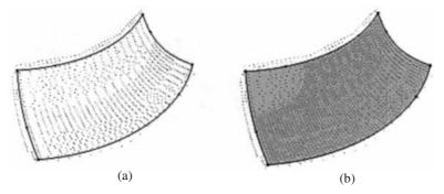
Figure 10.14 (a) Boundary B-spline curves with the segmented cloud (b) Coon's patch fit using the boundary curves
