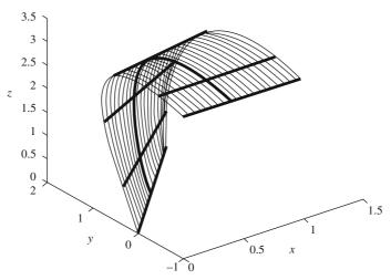
Figure 7.1 Example of a tensor product surface
