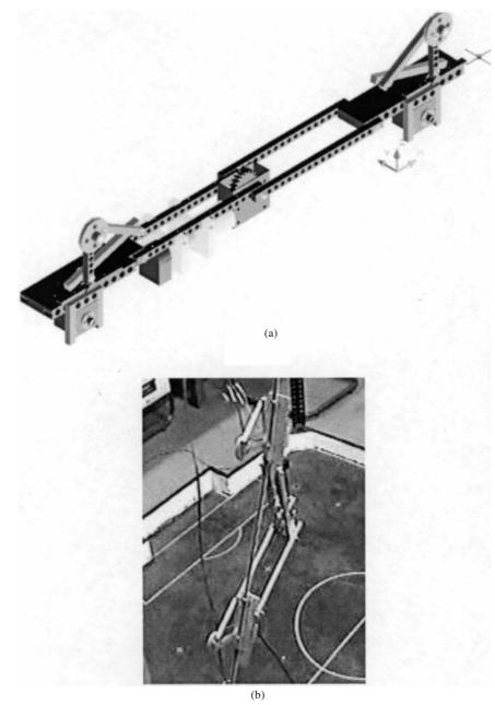
Figure 8.26 (a) CSG model of a Robosloth and (b) Robosloth in working
