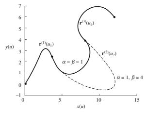
Figure 4.8 Example 4.4 for curve blending
