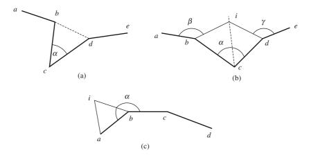
Figure A1.3 Advancing front method with various internal angles between consecutive edges of the front
