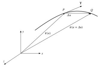
Figure 3.6 Parametric curve represented in vector form
