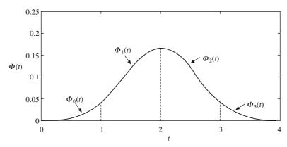
Figure 5.5 Computed normalized cubic spline with knots  $t_i = i$ ,  $i = 0, \ldots, 4$  for Example 5.2
