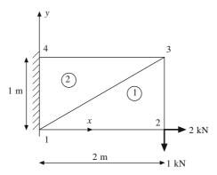
Figure 11.13 Displacement analysis of a rectangular plate
