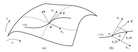
Figure 6.7 A curve c(t) on a parametric surface
