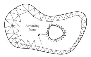
Figure A1.4 Schematic of the advancing front method
