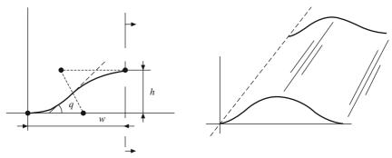
Figure P3 Cross section profile and the corresponding sweep surface. Input parameters for the cross section profile are (w, h and q). First find the position vectors  $r_0, r_1, r_2$  and  $r_3$  and then proceed.
