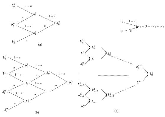
Figure 4.13 Triangular scheme for (a) n = 2, (b) n = 3 and (c) to compute intermediate de Casteljau points. Schema on top right is representative of the weighted linear combination of de Casteljau's points
