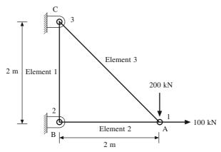
Figure 11.5 Truss assemblage for Example 11.1
