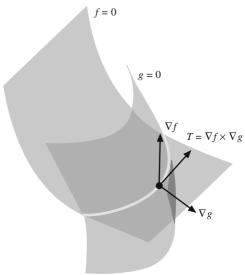
Figure 6.23 Curve of intersection between two surfaces
