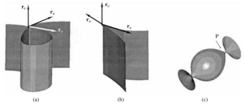
Figure 6.5 Singular points and lines on surfaces
