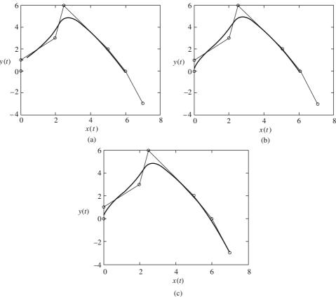
Figure 5.16 Unclamped and clamped B-spline curves: (a) unclamped spline, (b) spline clamped at one end and (c) spline clamped at both ends
