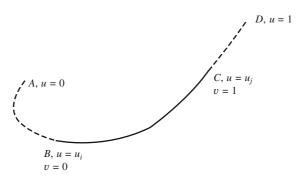
Figure 4.6 Trimming of a curve
