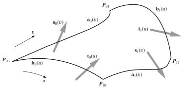
Figure 7.15 Schematic of a bi-cubic Coon's patch
