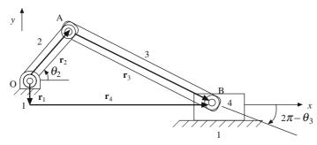
Figure 1.4 A slider-crank mechanism
