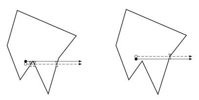
Figure 9.7 Crossings test for a ray passing through a vertex
