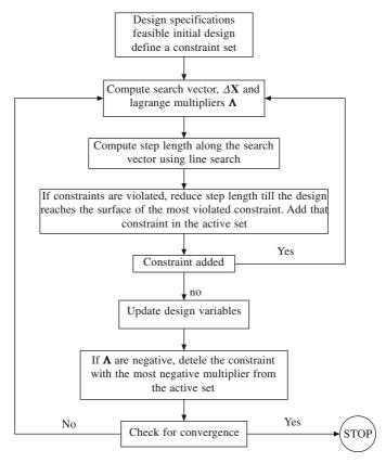
Figure 12.13 Implementation details for sequential quadratic programming
