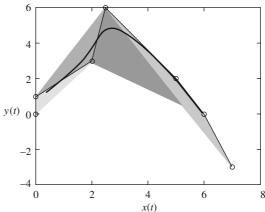
Figure 5.17 The convex hull property of B-spline curves
