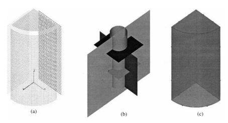
Figure 10.12 (a) Segmented cloud (offset), (b) algebraic surfaces fitted to segmented cloud and (c) solid model after intersection and trimming.
