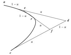
Figure 4.11 Geometric construction of a parabola
