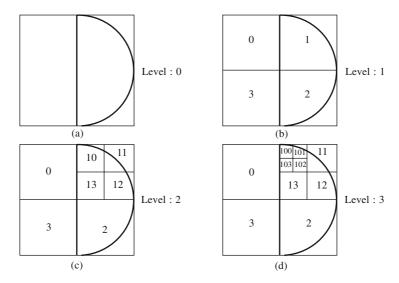
Figure 9.15 Quadtree decomposition of a semi-circular disc
