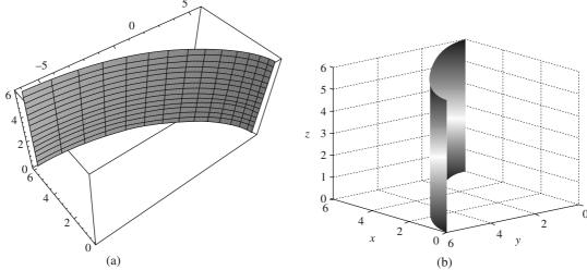
Figure 7.4 Ferguson patch for Example 7.2.
