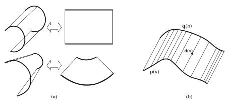
Figure 6.14 (a) Developable and (b) ruled surfaces
