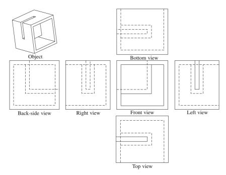
Figure 2.25 An object's orthographic projections in first angle
