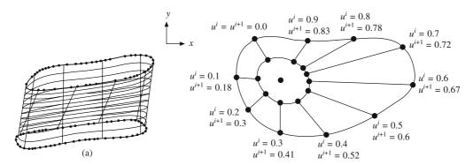
Figure 10.8 (a) A bad linear parameter correspondence leading to twisting and (b) parameter correspondence determined by angular spacing (viewing into the z direction)
