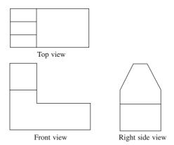
Figure 2.29 Three orthographic views in third angle
