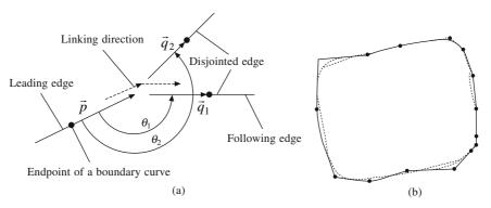
Figure 10.6 Edge tracking with edge points: (a) edge tracking illustrated at a point of branching and (b) illustration of closed B-spline contour fitting through the tracked edge points
