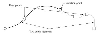
Figure 3.4 A schematic showing a composite curve with two cubic segments interpolating the data points
