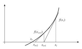
Figure 12.7 Newton-Raphson method
