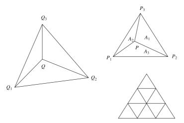
Figure A1.2 Structured triangular meshes
