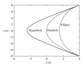
Figure 4.10 Conics with Ferguson's segments
