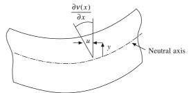
Figure 11.7 Axial displacement u in the beam
