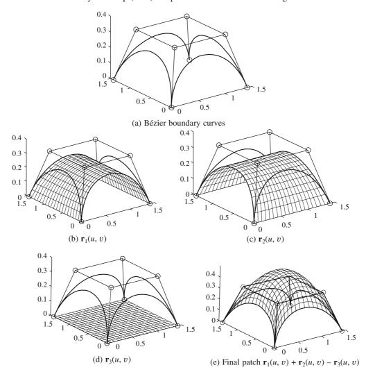
Figure 7.16 Bilinear Coon's patch in Example 7.8
