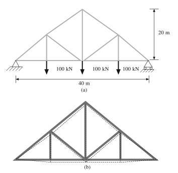
Figure 11.11 (a) An over-bridge modeled with frame elements and (b) displacement profile (scaled)
