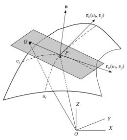
Figure 7.3 Tangent plane on the surface patch.
