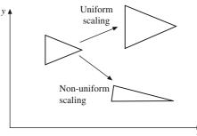
Figure 2.11 Uniform and non-uniform scaling
