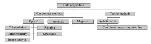
Figure 10.1 Data acquisition methods
