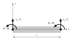
Figure 11.6 A beam element
