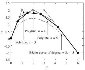
Figure 4.19 Degree elevation of a Bézier segment
