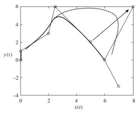
Figure 5.18 Local shape modification of B-spline curves
