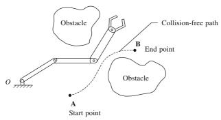
(b) Collision free path planning for a manipulator
