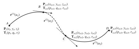
Figure 4.7 Blending of two Ferguson curve segments
