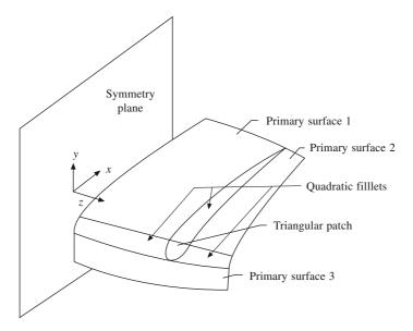
Figure P5 A scheme of surface patches for the automobile hood
