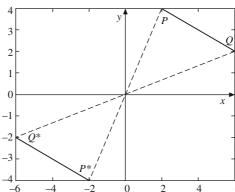
Figure 2.9 Reflection of a line through the origin
