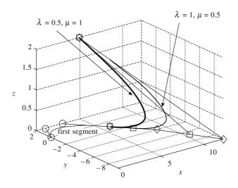
Figure 4.21 A  $C^2$  continuous composite Bézier curve
