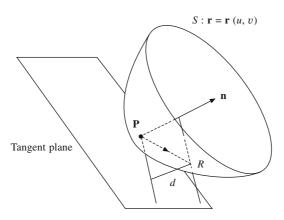
Figure 6.9 Deviation of R from the tangent plane
