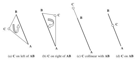
Figure 9.2 Proximity of a point and a line
