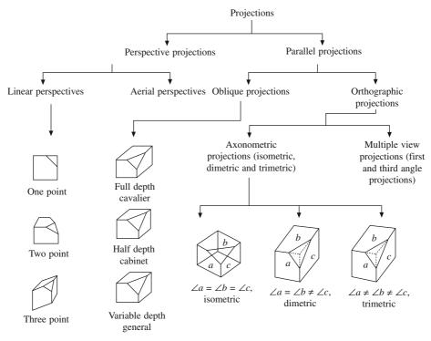
Figure 2.20 Classification of projections using a cube
