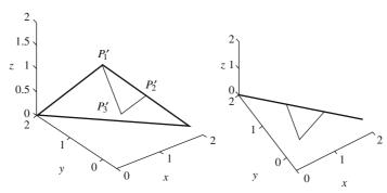
(e) Positions for case (iii), figure in right is edge view for  $Q_1Q_2Q_3$
