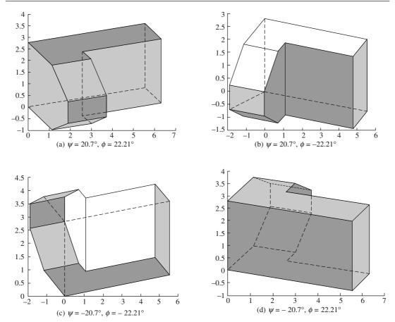
Figure 2.27 Four possible dimetric projections of the block
