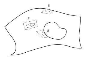
Figure 8.6 Boundary and interior points on the surface
