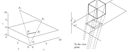
Figure 2.22 Perspective image of a line on the *x-y* plane in example 2.9
