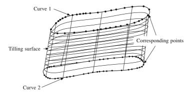
Figure 10.7 Linear parameter correspondence in tiling surface fitting
