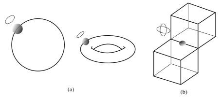
Figure 8.12 (a) Two-manifolds and (b) not a two-manifold
