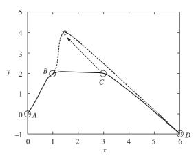
Figure 4.5 (a) Original (solid) and modified (dashed)  $C^1$  continuous Ferguson curves in Example 4.3 showing local control in shape change
