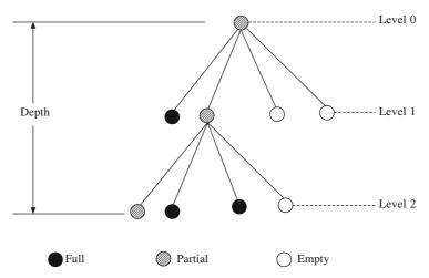
Figure 9.13 Schematic representation of a quadtree structure
