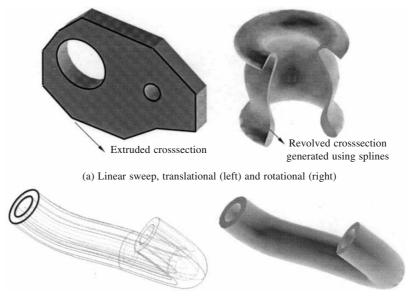
(b) Nonlinear sweep (wireframe in left showing crosssection and path)
