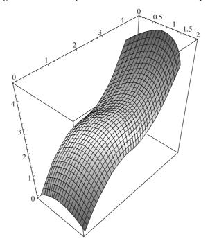
Figure 7.21 Composite bi-quadratic Bézier surface in Example 7.10
