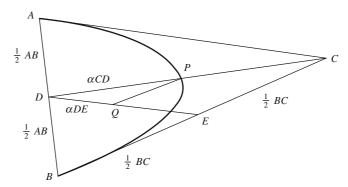
Figure 4.9 Construction for a conic section
