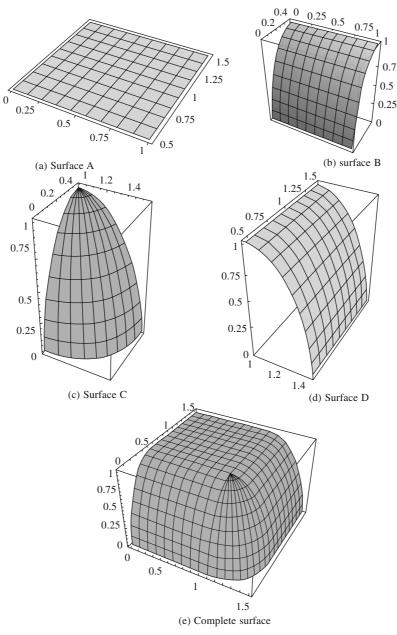
Figure 7.28 A Composite surface with four Coon's patches
