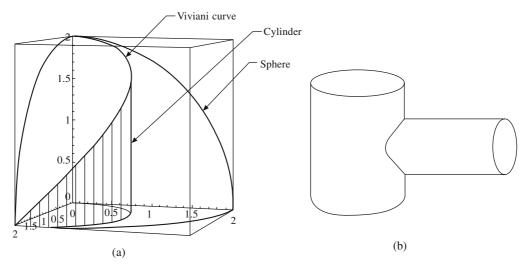
Figure 6.25 (a) Viviani curve and (b) intersection between two cylinders
