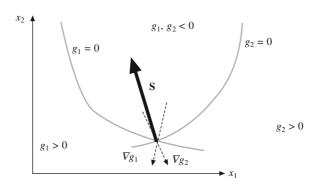
Figure 12.11 Geometric description of a feasible direction vector S
