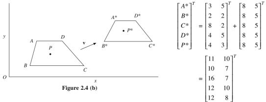
We may note that like rotation, translation as in Eq. (2.2) does not work out to be a matrix multiplication. Instead, it is the addition of a point (position vector) and a (free) vector. One may attempt to represent translation also in the matrix multiplication form to unify the procedure for rigid body transformations. Consider Eq. (2.2) rewritten as
