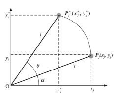
Figure 2.3 Rotation in a plane
