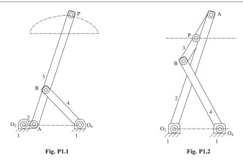
into the rectangular groove of the film, moves along a straight line by 35 mm and then lifts up to disengage from the film at the end of its motion. Design the mechanism by selecting suitable sizes of the linkages. Links 2 and 4 are parallel.
