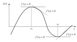
Figure 12.1 Optimality condition for a function of a single variable
