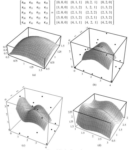
Figure 7.30 B-spline surfaces
