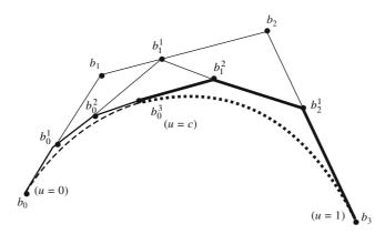
Control polylines for the two subdivided curves (thick and thicker solid lines) and subdivided curves (dashed lines)
