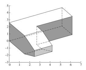
Figure 2.28 A trimetric projection of the block
