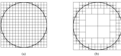
Figure 9.12 (a) A circular disc and its grid and (b) its quadtree decomposition
