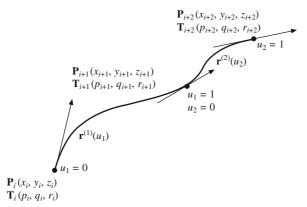
Figure 4.4 A composite Ferguson curve
