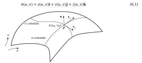
Figure 6.2 A parametric surface r(u, v)
