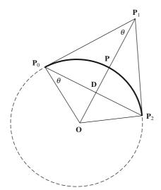
Figure 4.23 Design of a circular arc with rational Bézier curve
