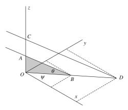
Figure 2.30 Geometry for oblique projections
