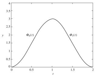
Figure 5.4 Plot of Splines  $\Phi_0(t) = 9t^2 - 6t^3$ ,  $0 \le t \le 1$  and  $\Phi_1(t) = 6t^3 - 27t^2 + 36t - 12$ ,  $1 \le t \le 2$
