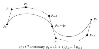
Figure 4.20  $C^0$  and  $C^1$  continuous Composite Bézice curves
