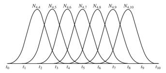
Figure 5.20 A schematic of cubic B-spline basis functions
