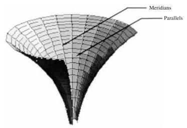
Figure 6.19 Funnel as a surface of revolution
