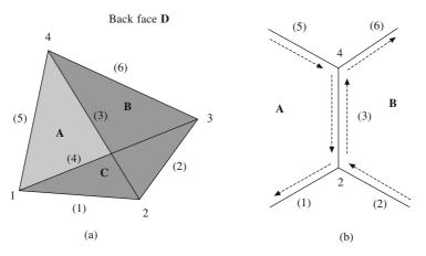
Figure 8.17 Winged-edge data structure for a tetrahedron
