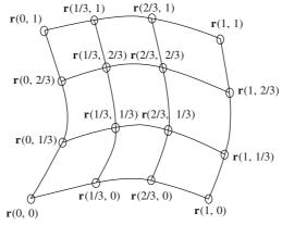
Figure 7.5 Bi-cubic surface patch in 16 point form
