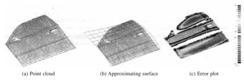
Figure 10.13 An approximating B-spline patch for a segmented point cloud.
