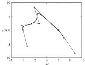
Figure 5.22 Interpolation with B-spline curves.
