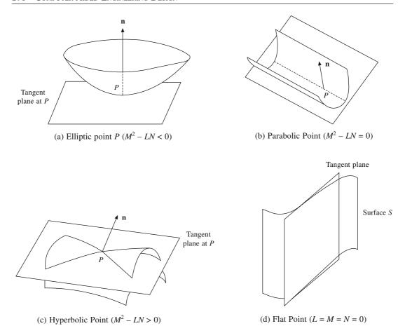
Figure 6.10 Classification of points on a surface
