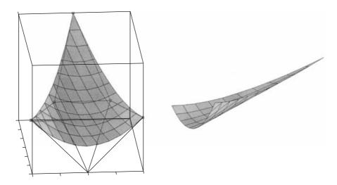
Figure 7.11 Triangular surface patch.
