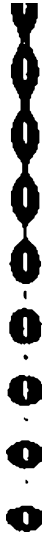
Fig. 4 Image of the drops generated by introducing an acoustic wave to the fluid stream. The break-off point is extremely stable allowing for the precise charging of individual drops and deflection of desired particles
