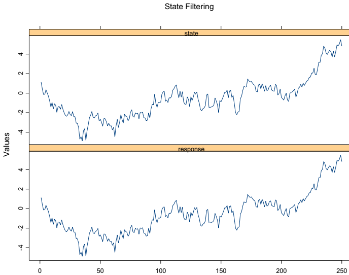
FIGURE 14.5. Filtered estimates of \alpha_t and y_t computed from simulated data from local level model.
