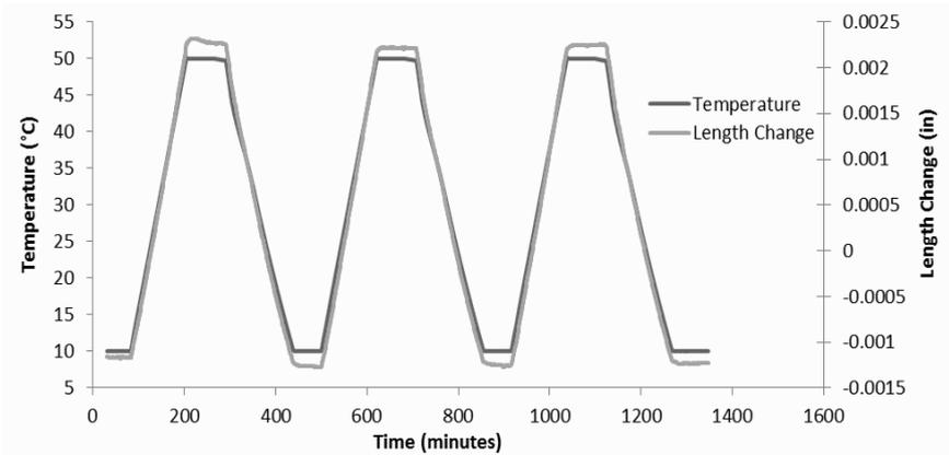
(b) Typical response of a concrete cylinder subjected to three heating and cooling cycles.
