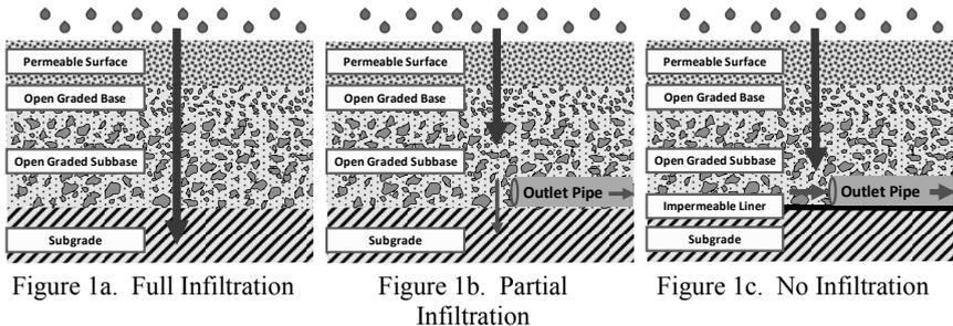
Figure 1a shows a full infiltration design. All stormwater is infiltrated into the subgrade below the pavement. This system does not require any additional stormwater features such as catchbasins, outlet pipes, stormwater management ponds, etc. This system is typically only used in areas where the subgrade materials have high infiltration rates.
