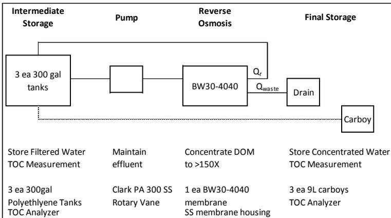
**Figure 2. Schematic view of the concentration process using one Filmtech BW30-4040 membranes.**
