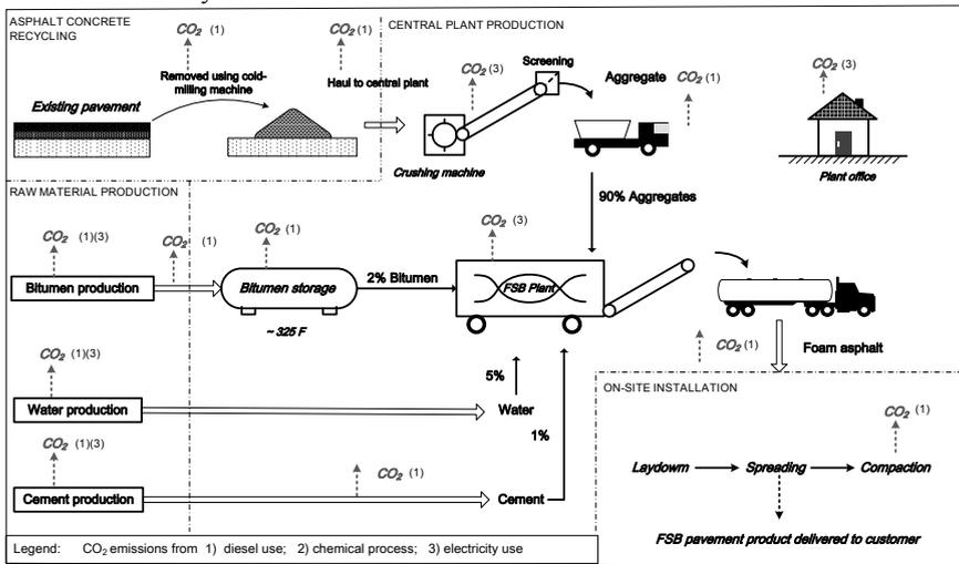
Fig.2 schematic of FSB pavement life cycle showing major system processes and emissions sources.
