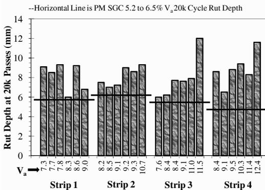
Figure 5. HLWT Test Results for HMA Strips 1 to 4
