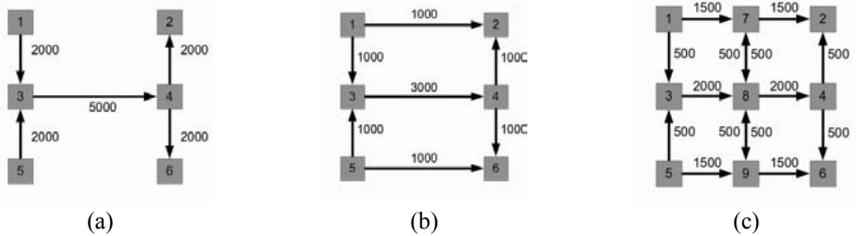
**Figure 3. Equilibrium flows for all three networks, accounting for signal retiming and drivers changing routes to be on shortest paths.**
