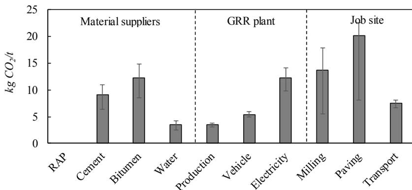
Fig.3. distribution of GHG emissions across the FSB pavement life cycle on a functional unit basis
