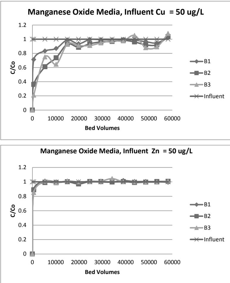
Figure 5. FBR breakthrough profiles for Cu(top) and Zn (bottom) from a synthetic stormwater solution onto granular manganese oxide (columns B1-B3 in series).
