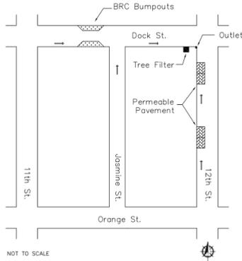
**Figure 2:** Layout of LID SCMs with arrows indicating direction of flow (not to scale)
