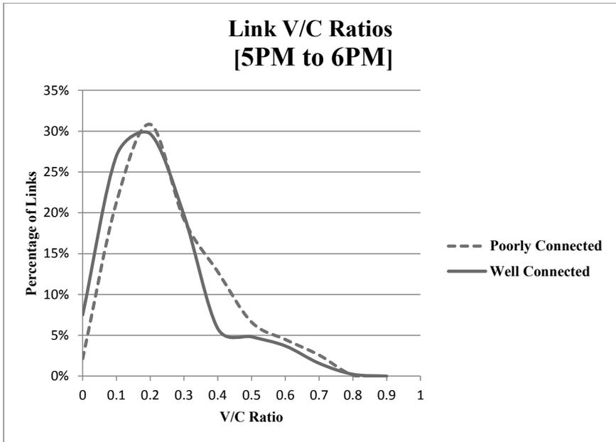
**Figure 8. Volume-to-capacity ratios on the links in the two scenarios.**
