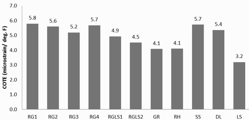
**Figure 2: Coefficient of Thermal Expansion (COTE) for concrete specimens older than 28 days.**
