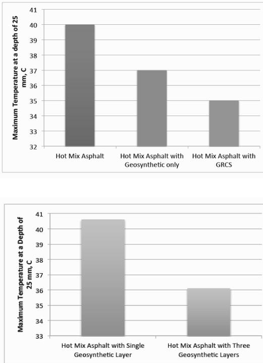
Figure 8. Results of experiments showing effect of chip seal and geosynthetic layer and thickness of geosynthetic layers
