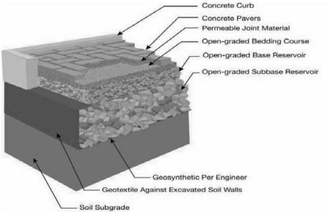
**Figure 4. PICP with full infiltration design.**
