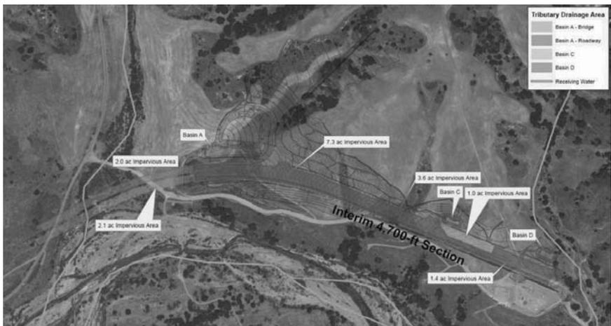
Figure 1 – Overview of New Project Drainage Area and LID Features
