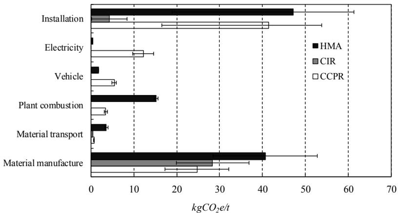
Fig.4. GHG Emission comparison amongst CIR, CCPR, and HMA base rehabilitation
