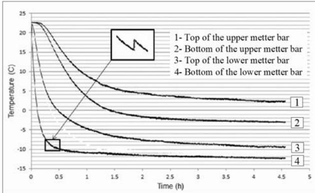
Figure 3. Data collected by the GLC for a system set to reach  $-20^{\circ}\text{C}$  as quickly as possible.
