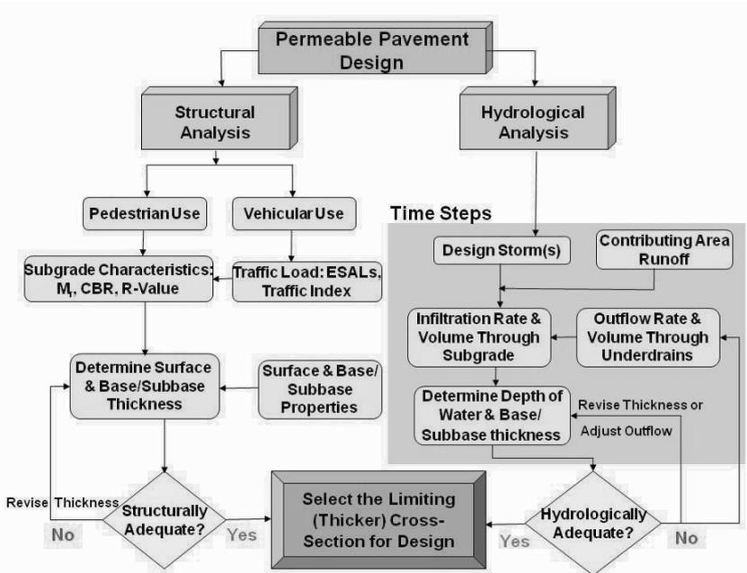
**Figure 7. Permeable pavement design flow chart (Smith 2011)**
