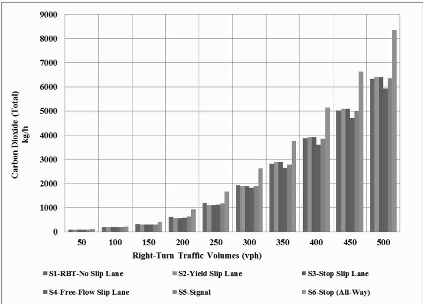
**Figure 4. SIDRA: Roundabout (Intersection) Total Carbon Dioxide (CO<sub>2</sub>) Emissions for Scenarios S1-S6.**
