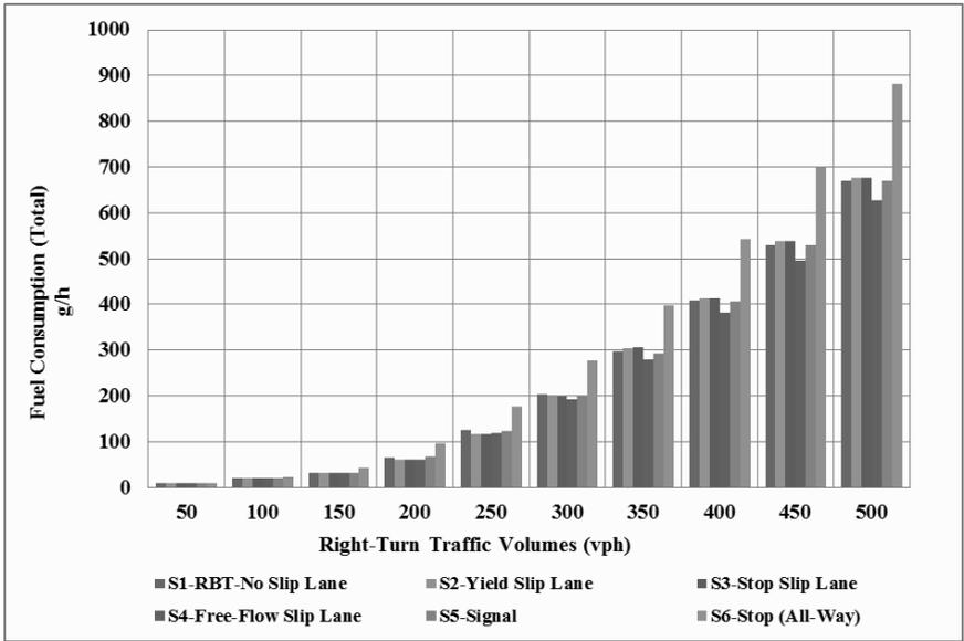
**Figure 3. SIDRA: Roundabout (Intersection) Total Fuel Consumption for Scenarios S1-S6.**
