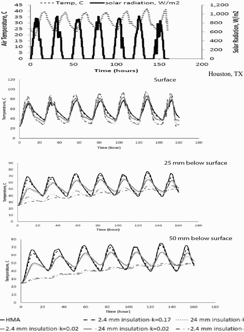
Figure 1. Air temperature and solar radiation, and results of simulation for Houston
