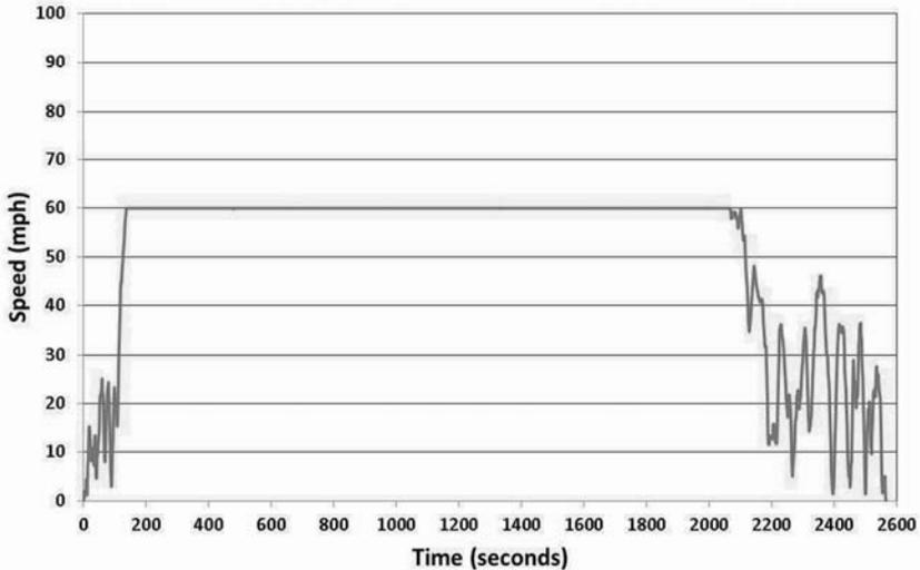
**Figure 6 Modified GRTA Xpress Cycle for Electric Vehicle Options**
