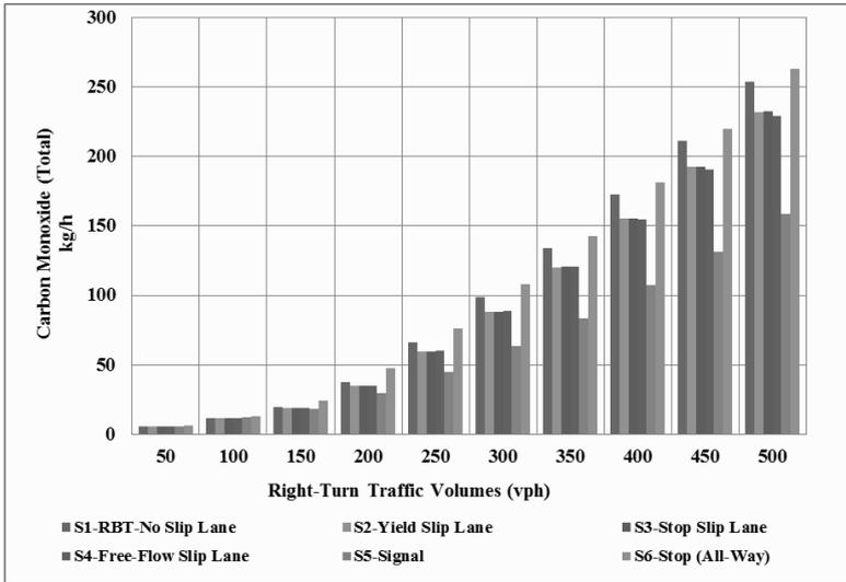
**Figure 5. SIDRA: Roundabout (Intersection) Total Carbon Monoxide (CO) Emissions for Scenarios S1-S6.**
