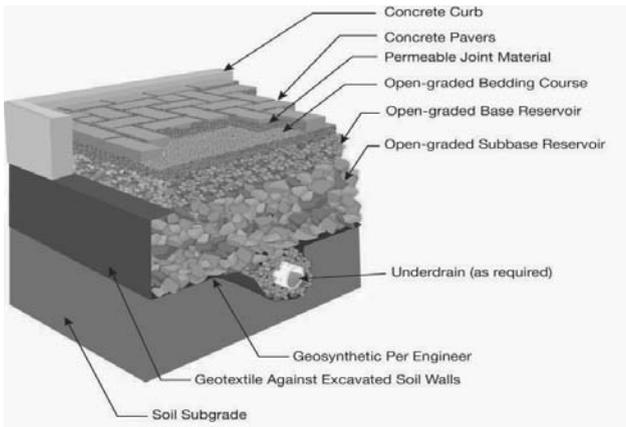
**Figure 5. PICP with a partial infiltration design using an underdrain.**
