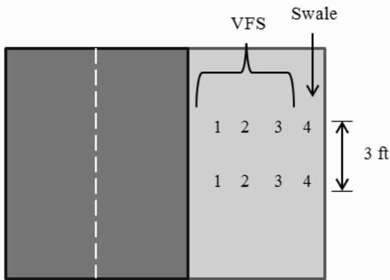
**Figure 2.** Site sampling regime, where position 1 is closest to the roadway. Positions 1, 2 and 3 constitute the VFS. Position 4 represents the swale or wetland swale. At each position two soil cores were taken at 0-0.1 m and 0.1-0.2 m depths. (not to scale)
