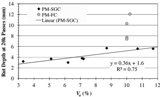
Figure 4. HLWT Test Results For Mix ID P
