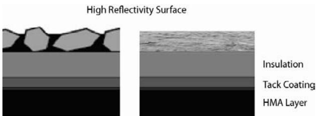
Figure 5. Desirable combination of high reflectivity surface and insulation near the surface
