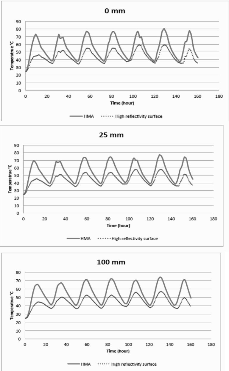
Figure 3. Effect of high reflectivity surface on the temperature
