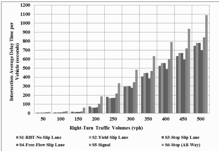
**Figure 2. SIDRA: Roundabout (Intersection) Average Delay for Scenarios S1-S6.**
