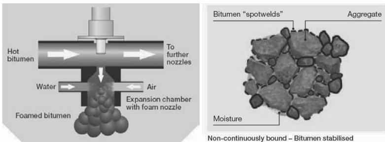
Figure 1 Foamed stabilized based process illustration and final product (Figure from Whirgen)
