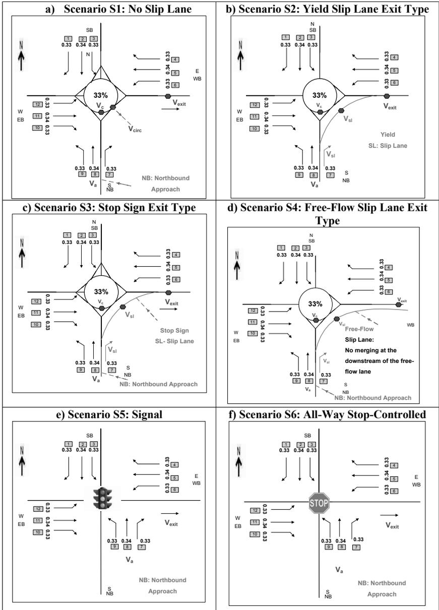
$V_a$  : Approach volumes.  $V_{exit}$ : Exit approach volumes.  $V_c$ : Conflicting circulating volumes.  $V_{sl}$ : Slip lane volumes as dominant right turn, vehicles per hour, for S1-S4.  $V_{cir}$ : Circulating volumes for S1-S4. Movement Turn No. 7 represents right turn, vehicles per hour, for S5-S6.
