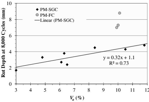
Figure 2. APA Test Results For Mix ID P
