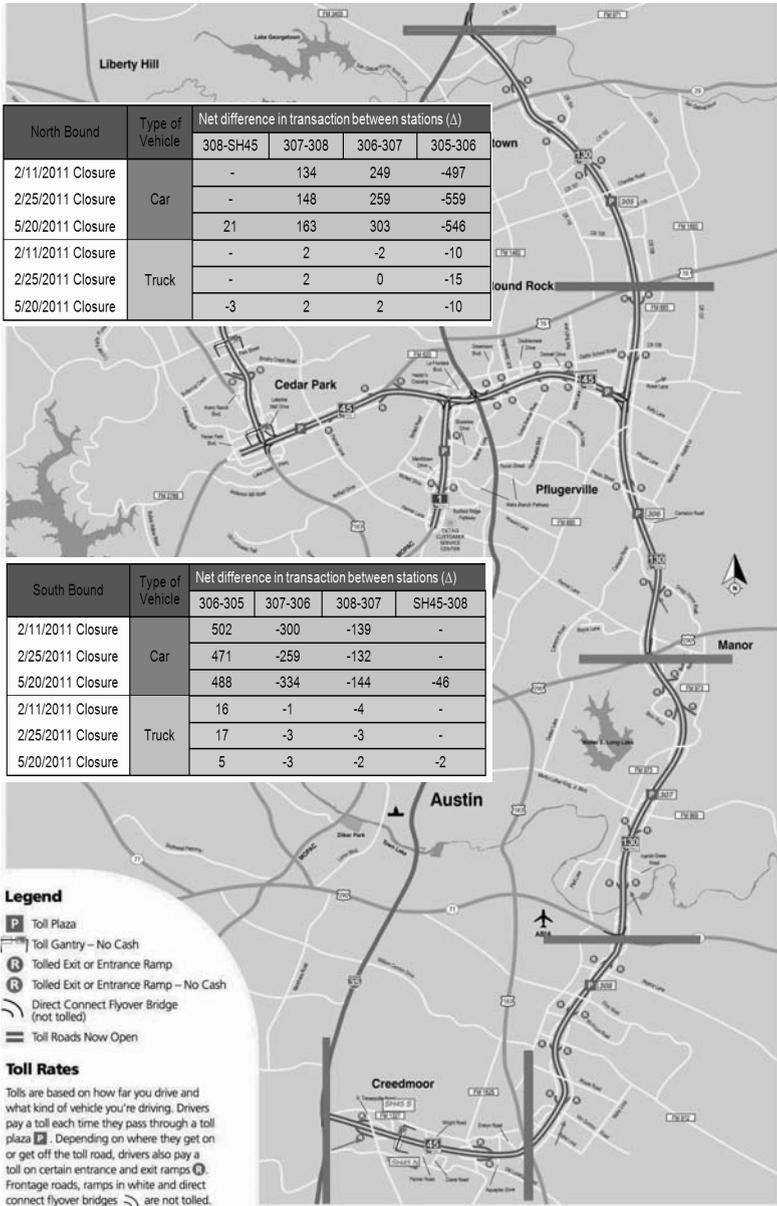
Figure 1: SH-130 segment/station descriptions and Net changes in southbound SH 130 traffic transactions among successive toll stations during closures
