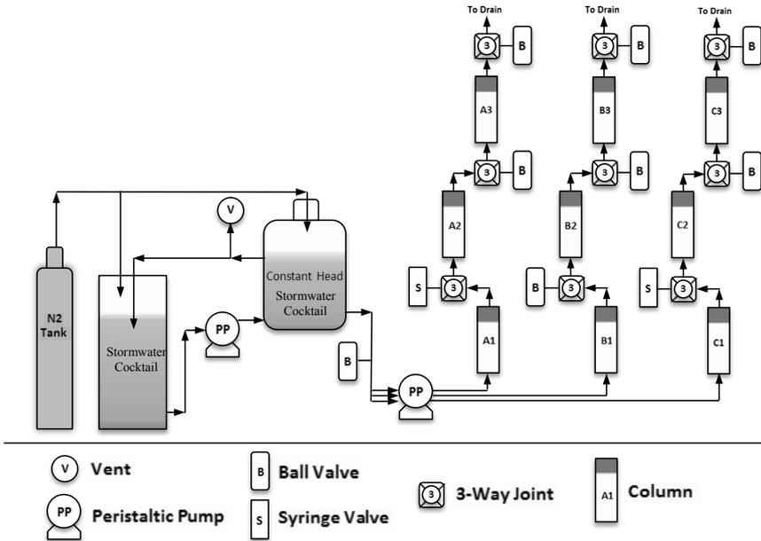
Figure 3. Experimental column setup (not to scale)
