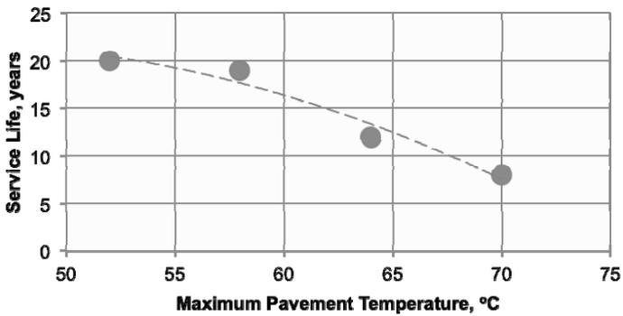
Figure 4. Service life versus maximum pavement temperature
