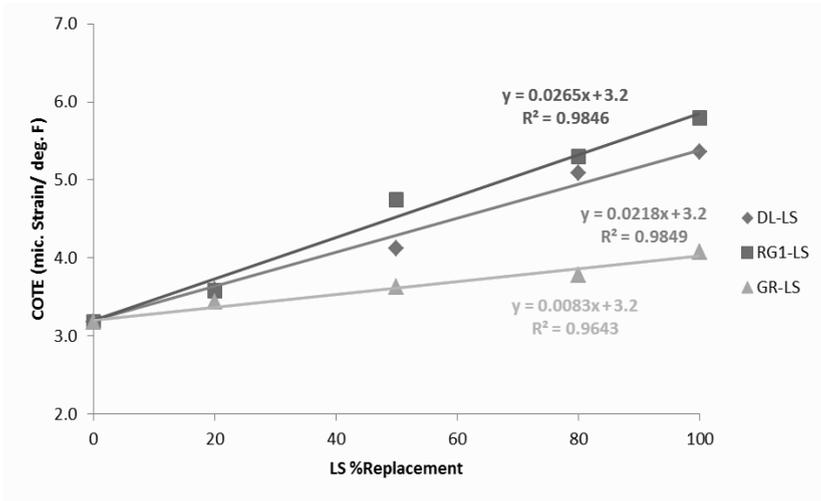
**Figure 3: Relationship of change in concrete COTE with limestone %replacement.**
