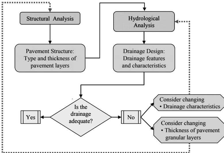
Figure 2. Structural and hydrological design flowchart [Swan 2009].
