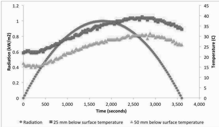
Figure 4. Data collected from the Solar Simulator for a hot mix asphalt sample.
