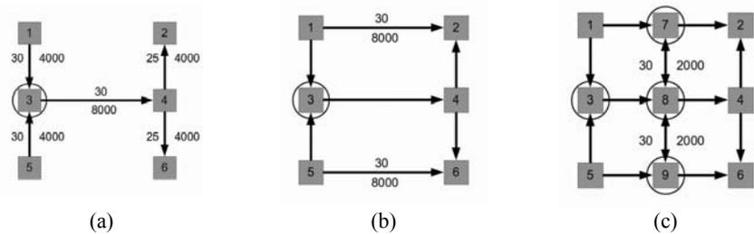
**Figure 2. Three networks demonstrating non-monotone relationship between connectivity and mobility. Figures indicate new links' speed limit (mph) and saturation flow (vph).**
