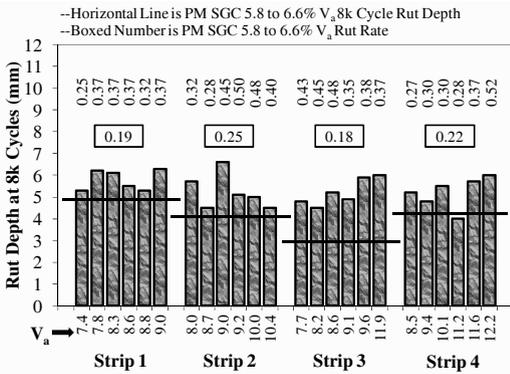
Figure 3. APA Results for HMA Test Strips
