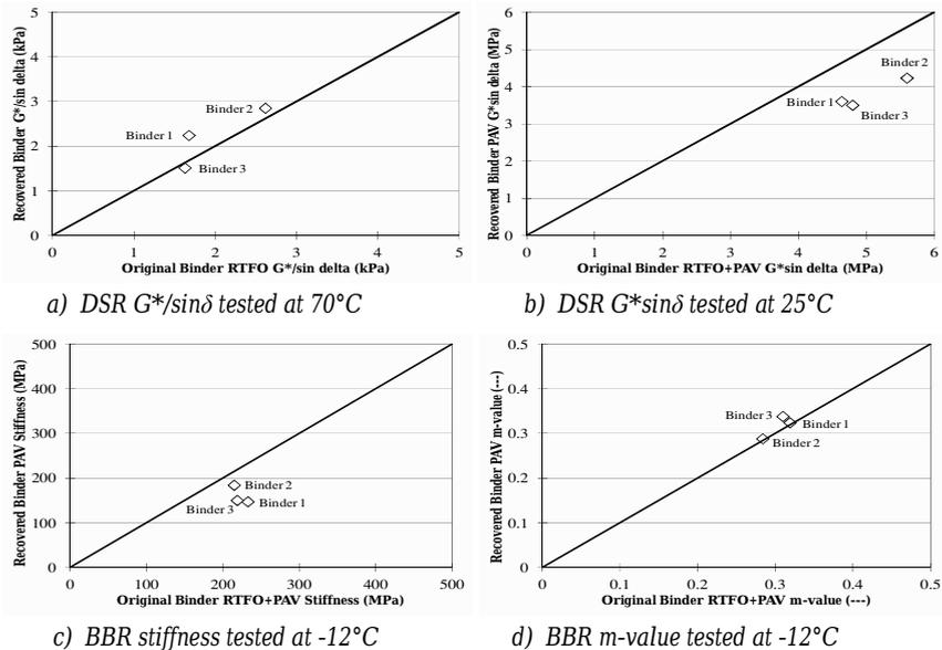
**Figure 4. Original and Recovered Binder Raw Test Data Comparison**
