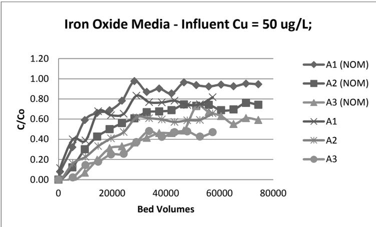
**Figure 6. Comparison of FBR breakthrough profiles for Cu from synthetic stormwater solution with and without reconstituted highway organic matter (NOM).**
