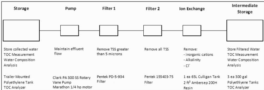
**Figure 1. Schematic diagram of the organic matter pretreatment process using filtration and ion exchange. Specific brands of equipment are provided as examples.**
