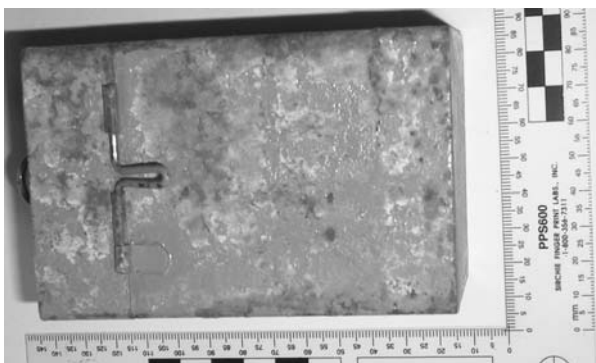
Figure 17: Dimensions of mustard gas container
