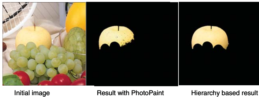
Fig. 25. On the left, initial image ; center: all pixels which are within a colour tolerance of an initial pixel. On the right, result of the magic wand.
