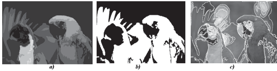
Fig. 10. a) Segmentation of the saturation (presented in grey tones); b) optimal threshold of a); c) final synthetic partition, superimposed to the initial image.
