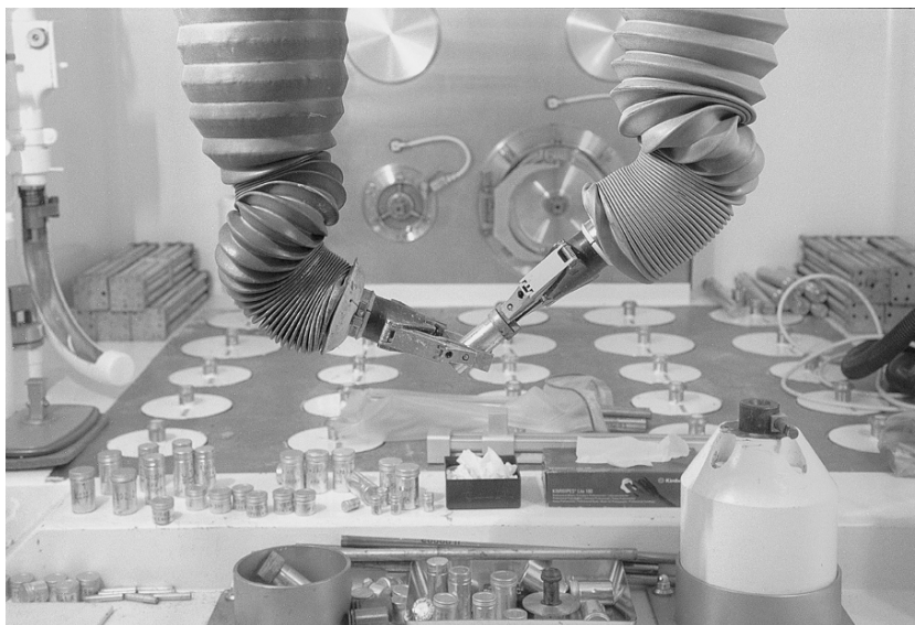
Fig. 1.4 Example of an experimental setup within a hot-cell facility. (Reproduced by permission of Institute for Transuranium Elements, Karlsruhe, part of the Joint Research Centre, European Commission.)
