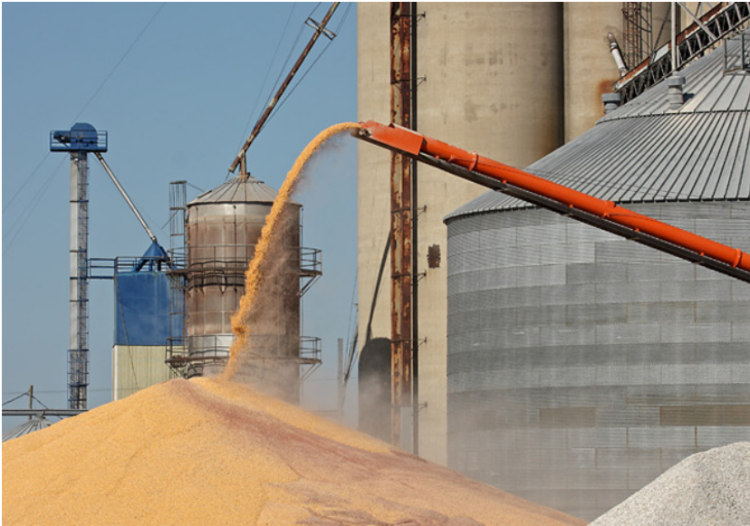
FIGURE 3.4 A common style of elevator in the U.S. These elevators are commonly constructed of steel and concrete. Worker exposure to grain dust is apparent in this photograph, and can be more concentrated in enclosed spaces. (Source: Charles Brutlag/Shutterstock.com.)
