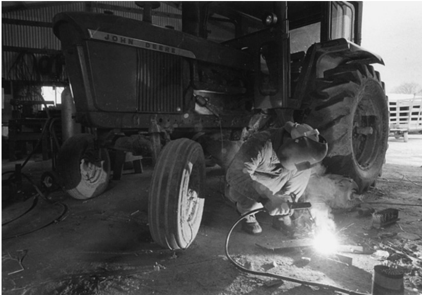
FIGURE 3.9 Welding is commonly practiced on many farms and may create a risk for metal fume fever, skin burns, and retinal inflammation.
