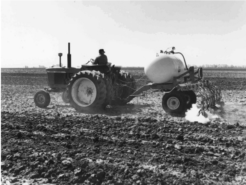
FIGURE 7.5 Anhydrous ammonia is an important fertilizer in many areas of the world. Excess nitrogen can run off with soil erosion, escape into the air, and be a source of chemical damage to the eyes and respiratory tract of applicators. (Note that this farmer is operating a tractor without a rollover protective structure. Injury from a possible overturn of this tractor is a much greater immediate risk to life than the anhydrous ammonia he is applying.) (Source: Medical Practice in Rural Communities , Chapter 3, Figure 3.4, page 46, book authors: Cornelia F. Mutel, Kelley J. Donham, Rural Health and Agricultural Medicine Training Program, Department of Preventive Medicine and Environmental Health, College of Medicine, The University of Iowa, Iowa City, Iowa 52242, U.S.A., © Springer-Verlag New York Inc., 1983. Image reprinted with kind permission of Springer Science and Business Media.)
