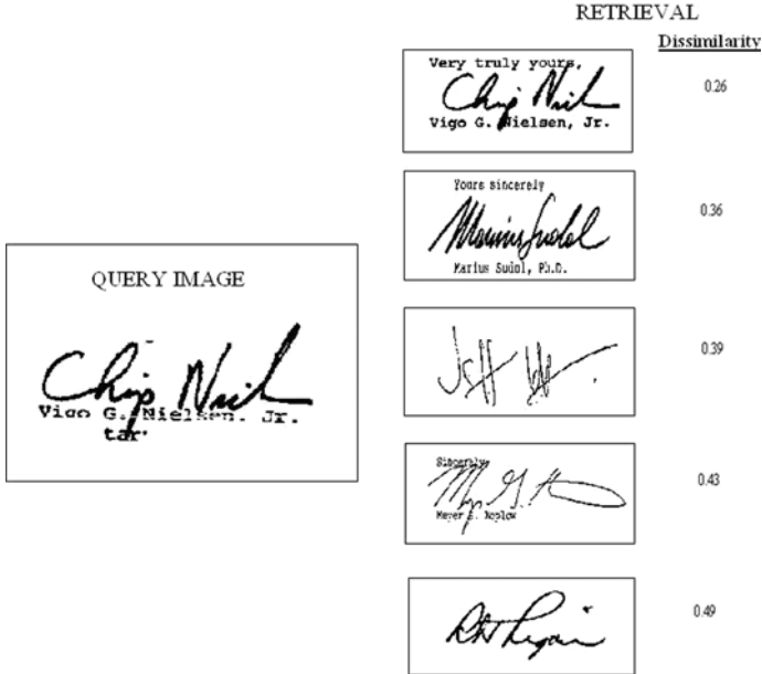
Fig. 2.6. Subset of retrieval results with the query image on the left and the signatures matched against and their corresponding dissimilarity distances on the right.
