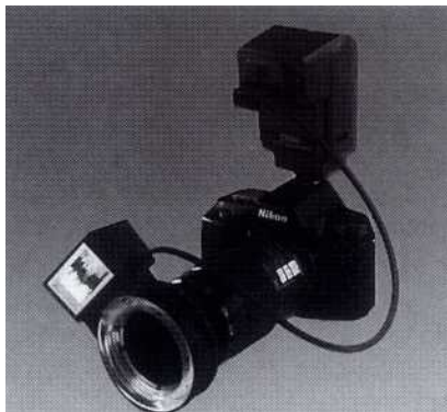
Fig. 14-7. Lester Dine Nikon N70 body with a modified Kiron 105-mm lens with both a point source and a ring light.
