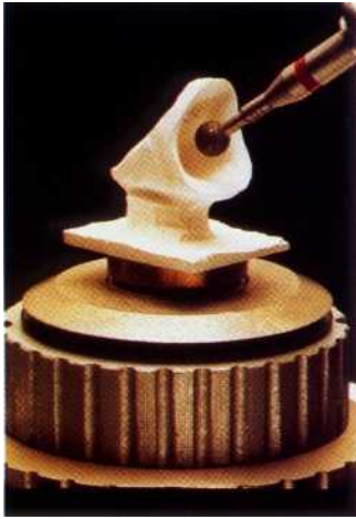
Fig. 24-26. Crown being fabricated by the Celay system. (Courtesy Vident, Inc.)
