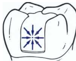
Fig. 5-4. Chemically cured composite resin shrinks toward the geometric center of the mass. (This may only occur if the composite is not bonded. Versluis thinks that composites shrink toward the adhesively bound surfaces.) This process leaves a small contraction gap at the gingival margin. The composite resin is strongly bonded to enamel on the buccal and lingual walls, preventing the formation of gaps at these walls; however, stresses may be set up in the tooth and the composite resin.
