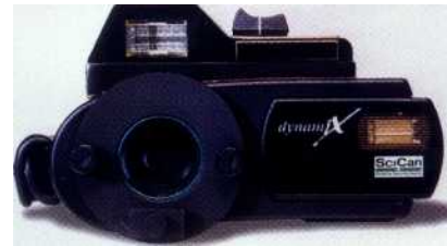
Fig. 14-11. A digital camera modified for dental use. (Courtesy SciCam, Inc.)
