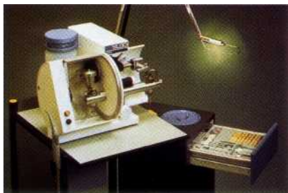
Fig. 24-27. A porcelain blank is milled into a porcelain restoration using an "eight axis of freedom micro-milling machine." (Courtesy Vident, Inc.)
