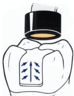
Fig. 5-5. Photocured composite resin shrinks toward the light source because the composite resin closest to the light hardens first. This pulls the softer composite resin from the gingival areas, creating a gap. The mass of composite resin being pulled to the occlusal area is twice that found in chemically cured resins (see Fig. 5-4); therefore the gingival contraction gap is roughly twice as large. Versluis thinks that composites shrink toward the adhesively bound surfaces. However, if the contraction is toward bound surfaces and not toward the light, this would not occur.
