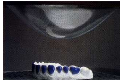
Fig. 13-22. The tray material is heated on a vacuum former unit. (Courtesy Ultradent Products, Inc.)
