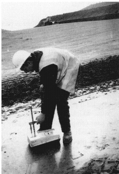
Figure 4 Use of nuclear density meter
